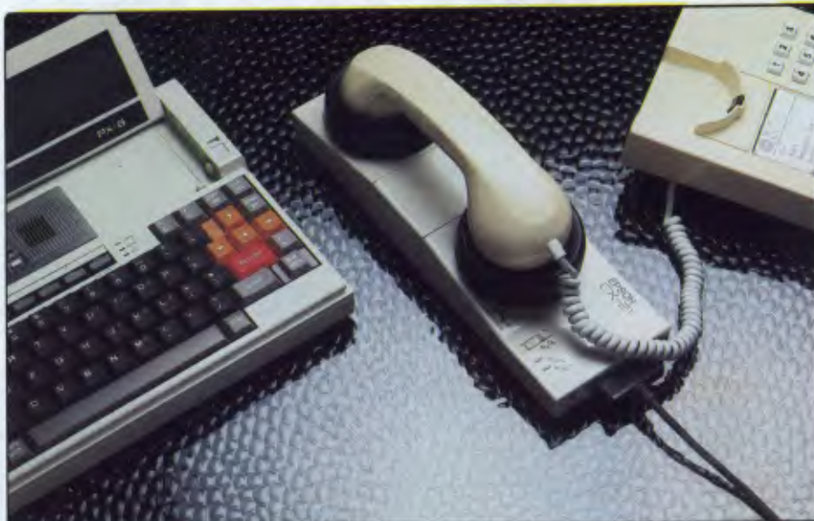
The CX-21 acoustic coupler can be used with the PX-8's TERM program
