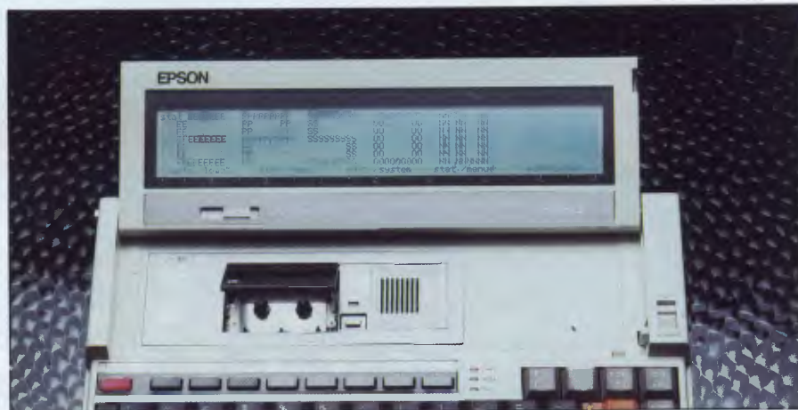
A ratchet mechanism allows the display to be set to various angles
