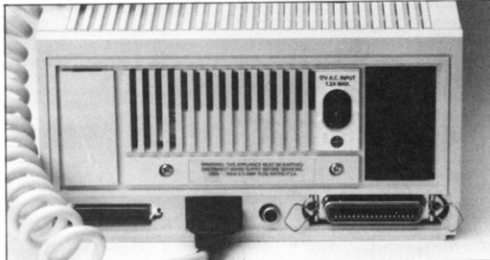
Although the monitor takes its power from the rear of the machine two power supplies are needed.
