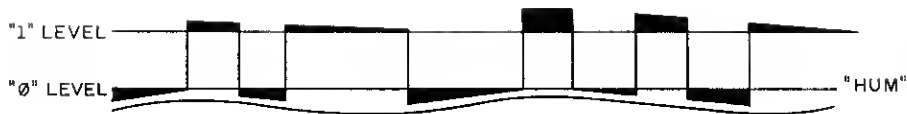
Fig. 1 Left. Exaggerated depiction of data pulses "riding" on the hum signal induced by ground loops between the TRS-80 and the cassette machine.
