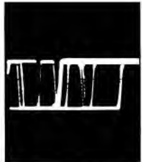
Photo 5. Speed fluctuations drive the syncing process to its limit. This signal was measured at the same point as in Photo 4.
