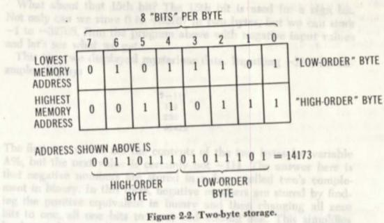
The first byte is the low-order byte, while the second byte is the high-order byte. This arrangement is true for all byte storage in the TRS-80 and is shown in Figure 2-2 for various values. We can see this better if we use some additional code to recompute the input value from the two bytes at which we've PEEKed.
