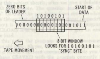
Figure 9-3. Synchronization operation.
