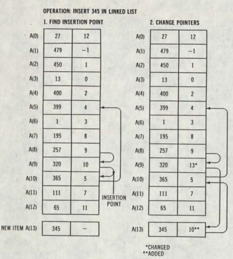
Figure 7-14. Insertion using linked list.
