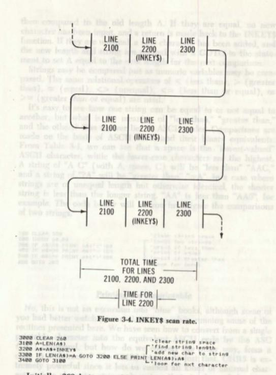
Initially, 260 bytes are CLEARed for string space to permit a maximum string length of 255 bytes to be created. Variable A is set equal to the length of the A\$ string, which is initially 0. (The LEN function returns the current length of a specified string.) Next, the INKEY\$ function is used to concatenate any keyboard character input. If none is input, A\$ is the same as before the INKEY\$ operation, as is the LENgth. The new length of A\$ is
