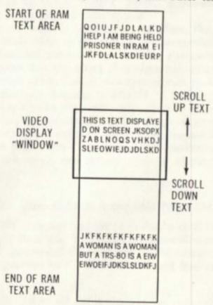
Figure 3-11. Text editing using display memory.
