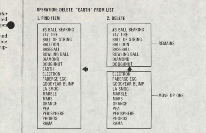
Figure 7-12. Deletion algorithm.
