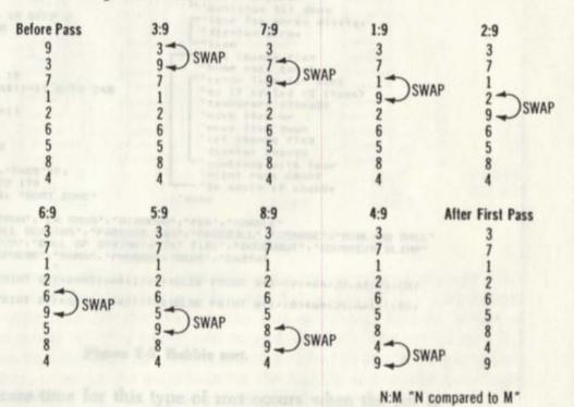
Figure 7-7. Bubble-sort algorithm.
