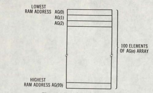
Figure 6-4. Example of one-dimensional array.
