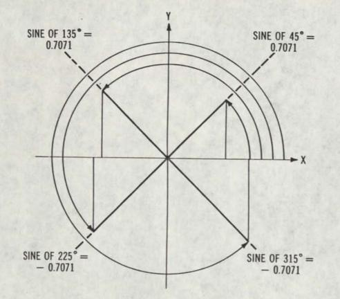
Figure 8-6. Sine function through 360°.
