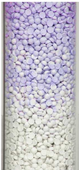
Top: exhausted CO 2 -X-Globuli; bottom: new material
