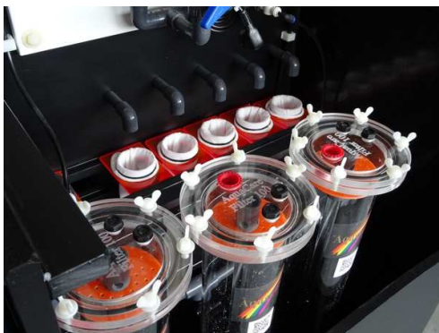
Several filter socks in a larger system with each associated inlet
