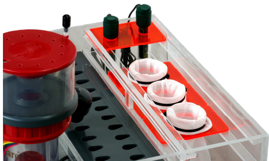
1.+2. chamber with holders for heating and measuring sensors, overflow screen for degassing stage, inlet from skimmer
