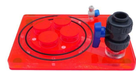
The effective inlet system for the formation of a fluidized bed
