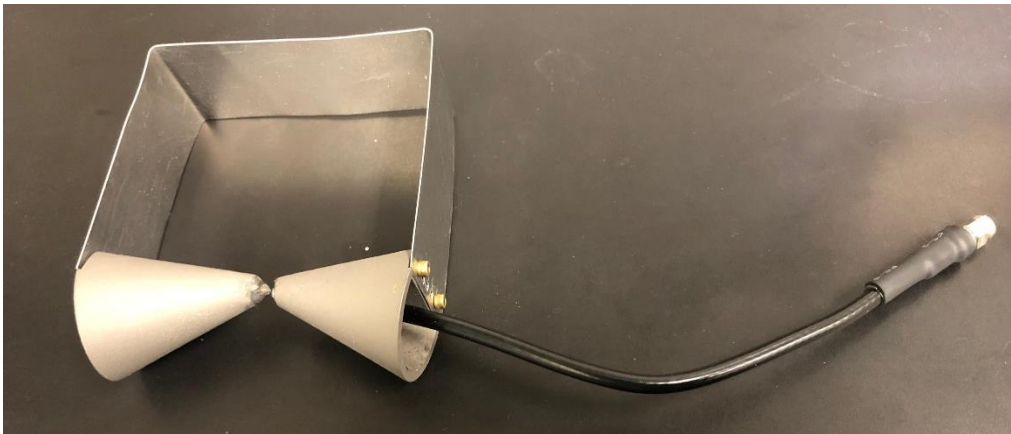
Figure 10.3.1. 3D printed and metallized prototype of single element Shark antenna.
