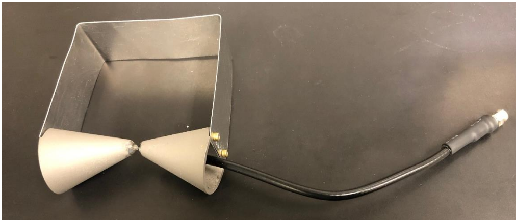
Figure 9.3.1. 3D printed and metallized prototype of single element Shark antenna.
