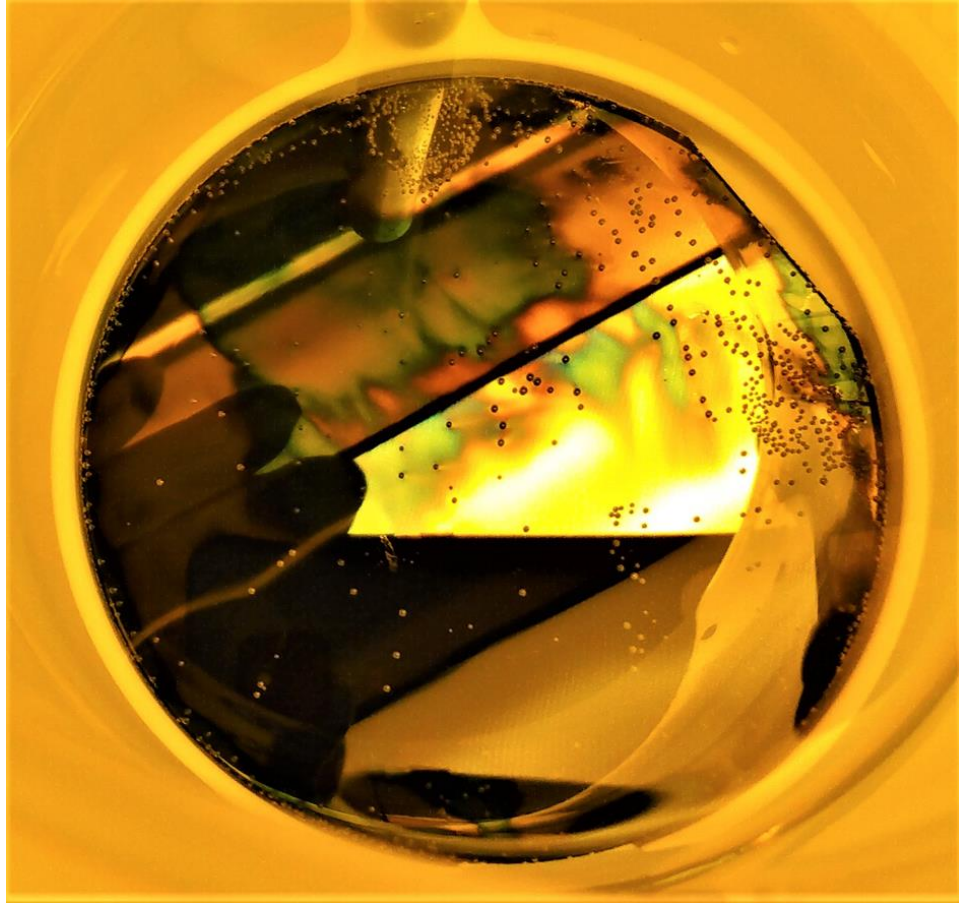
Figure 5.2.3. Hydrogen bubbles stuck to wafer surface in 1000:1 HF:HNO 3 recipe modified with a few drops of Triton-100.
