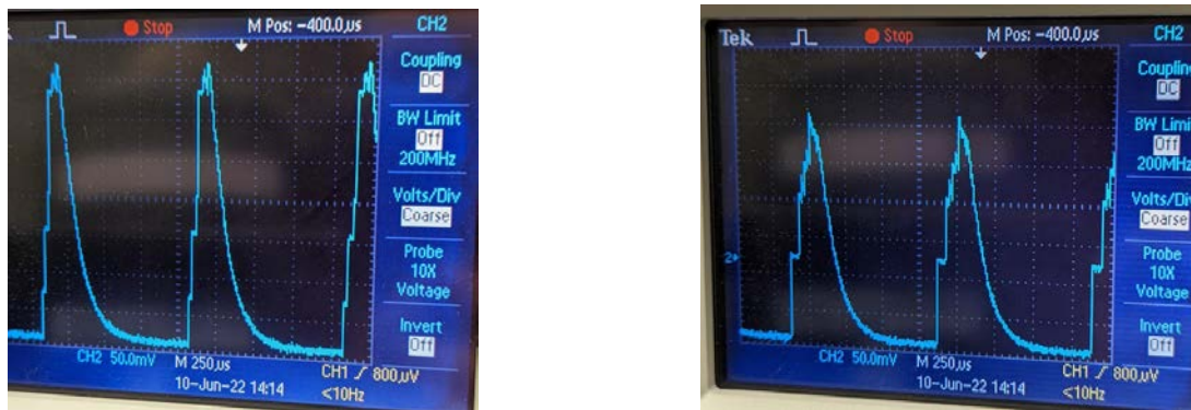
Fig. 3.1.1. Sample of scope traces demonstrating good pulse shape on the left and gain fluctuations on the right.
