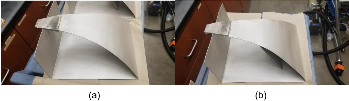
Figure 8.2.1. Two halves of the silver painted Koshelev antenna ready for assembly. (a) Bottom half and (b) Top half.
