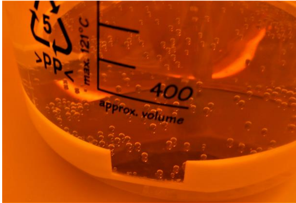
Figure 5.2.1. Control sample: wafer in beaker with 1000:1 HF/HNO 3 mixture. The hydrogen bubbles stuck to the wafer surface are clearly visible.
