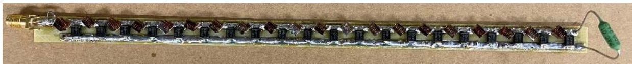
Figure 8.1.1. 20 cell D-NLTL of dimensions 1.1 x 23.45 cm constructed with commercial off the shelf components.
