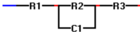
Figure 5.3.6. Equivalent circuit of DSRD as plotted in Figure 5.3.5.
