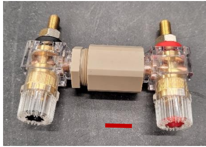
Figure 5.3.1P Press pack fixture that was used to collect current-voltage measurements from both the 371A curve tracer and from the Keithley picoammeter. This fixture applies consistent pressure across the diode and is expected to significantly reduce the variation found within the current-voltage measurements.
