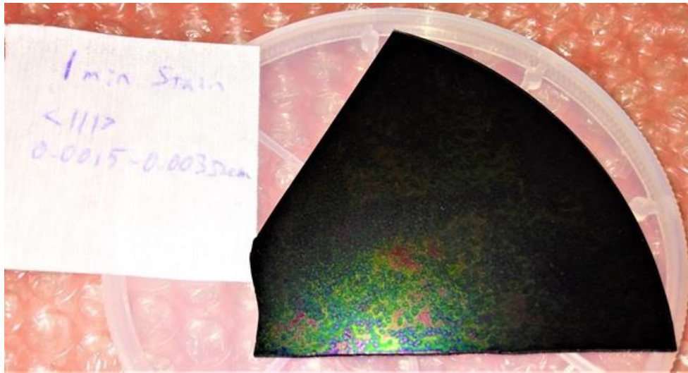
Figure 6.2.3. Example of stained silicon wafer.
