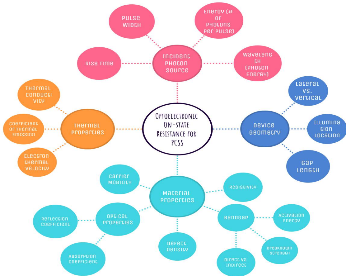
Figure 5.1.1. Chart of parameters affecting on-state resistance in PCSS, which will be iterated upon as the literature study progresses.
