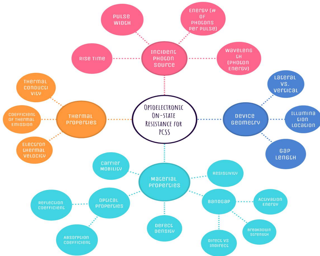
Figure 5.1.1. Chart of parameters affecting on-state resistance in PCSS, which will be iterated upon as the literature study progresses.
