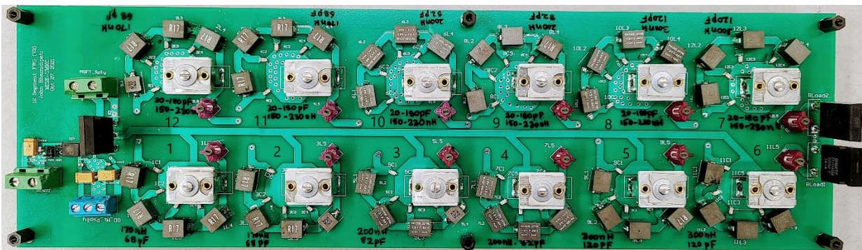
Figure 4.2.1. 12-segment lumped-element-based dynamically tunable FWG prototype with one pair of tunable L–C components per transmission line.
