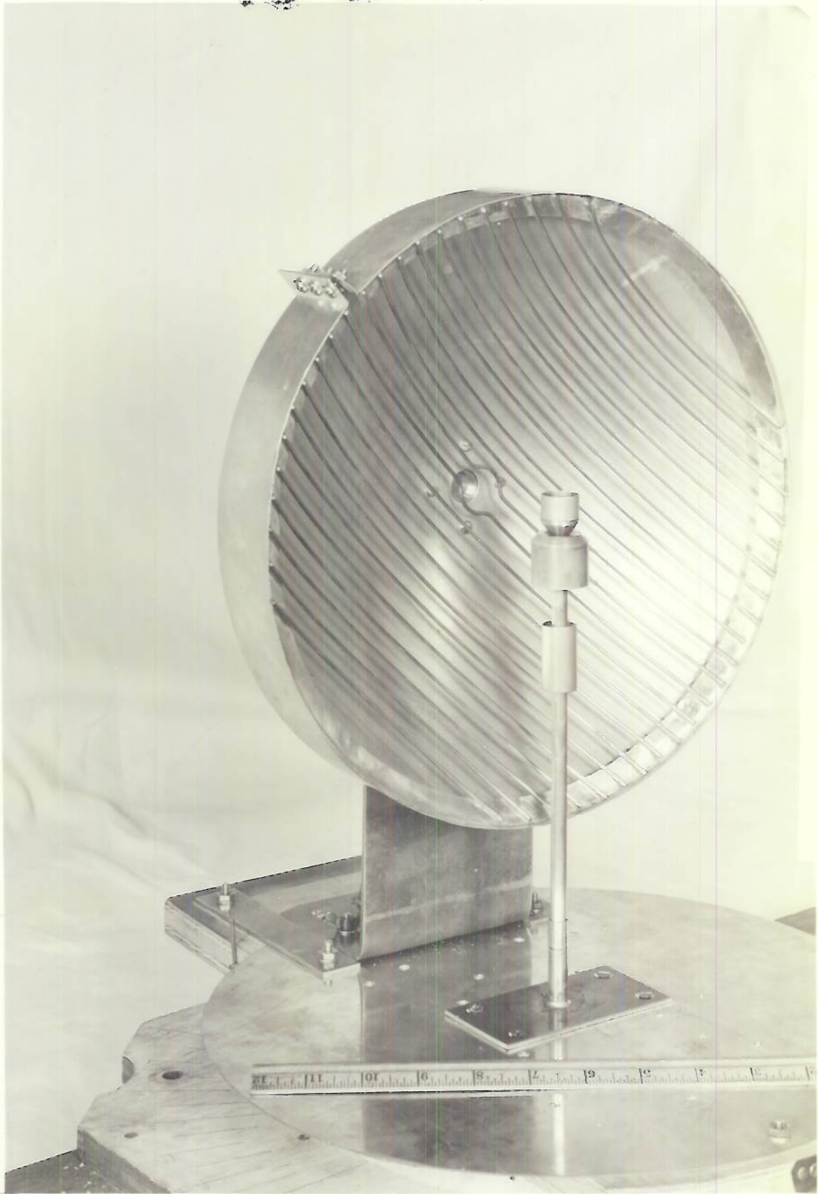
CIRCULARLY POLARIZED ANTENNA FED FROM BELOW.
