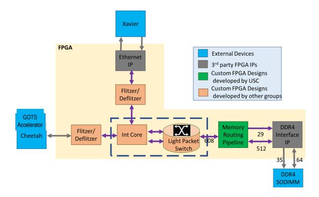
Figure 2. Top level model of FPGA design
