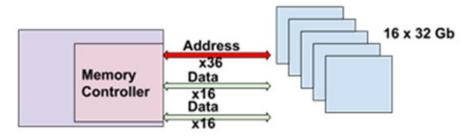
Figure 4. Memory design using 16 x 4 GB DRAM chips
