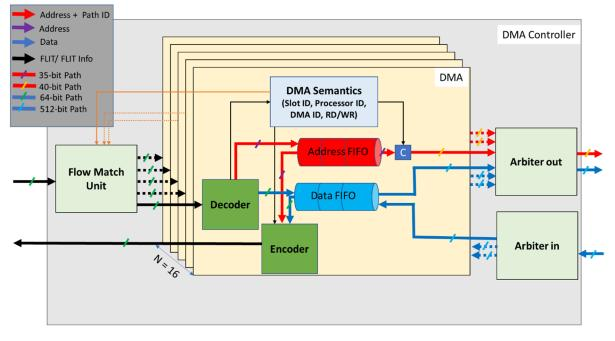
Figure 10. Overall architecture of DMA engine
