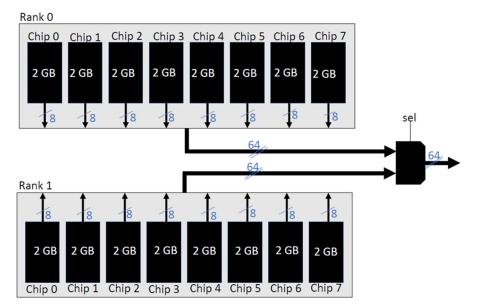
Figure 7. Internal structure of selected DDR4 SO-DIMMs
