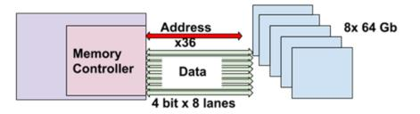
Figure 5. Memory design using 16 x 4 GB DRAM chips
