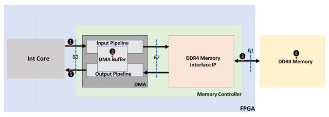
Figure 8. Conceptual design of the FPGA memory controller
