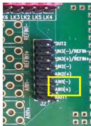
Figure 18. The AD7792/7793 demonstration board analog input pin connection.
