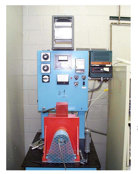
High-speed 203 bearing test 4 hr at room temp, 21 hr at 115°C, 1769 N load, As received grease and after 6 mo. storage at 71°C and 98-100% RH
