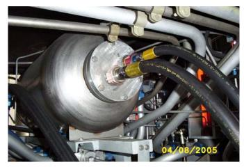
Hydraulic Reservoir End View New Manufactured End Cap Installed
