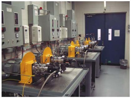
Six additional test heads added to existing 8 Will be used for oil-bearing life testing
