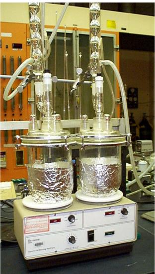
Corrosion Rate Evaluation Procedure Coupons, 300M steel, distilled water, 45 min.
