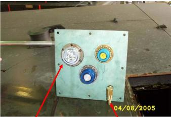
Unvented Filler Cap Vent Dryer Fitting
