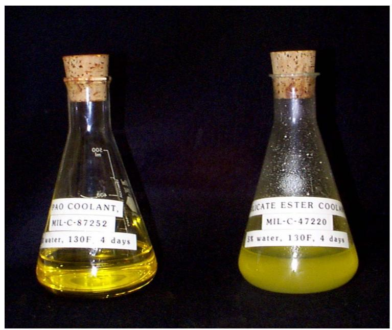
Hydrolysis study: MIL-PRF-87252 vs. silicate ester
