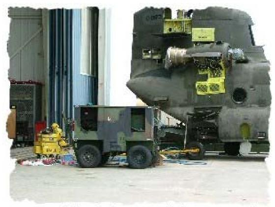
An aircraft hooked up to a mule (servicing cart), which is also hooked up to a purifier for a test.
