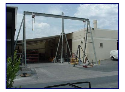
225 Ton Dynamic Hydraulic Jack Test Fixture
