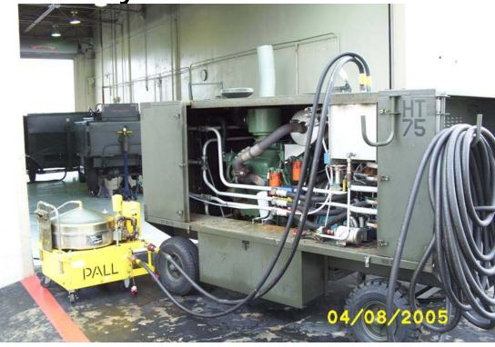
Vent Dryer Mounted On Inside Wall Of HTS Pall Purifier Hooked Up To HTS
