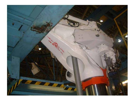
Landing Gear parts are given cadmium, IVD, phosphate, and paint for protection against corrosion.
