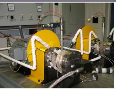
Bearing test heads with insulated head and oil supply lines for high temp operation
