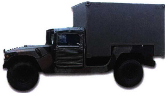
Figure 1. Lightweight, Rigid-Wall Shelter Mounted on a HMMWV
