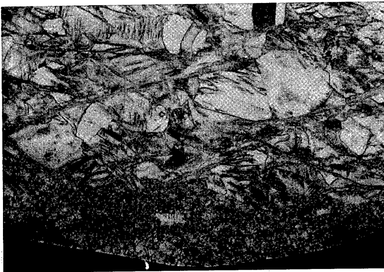
Figure 5: Microstructure of nitrogen alloyed steel with heat-affected zone. x200
