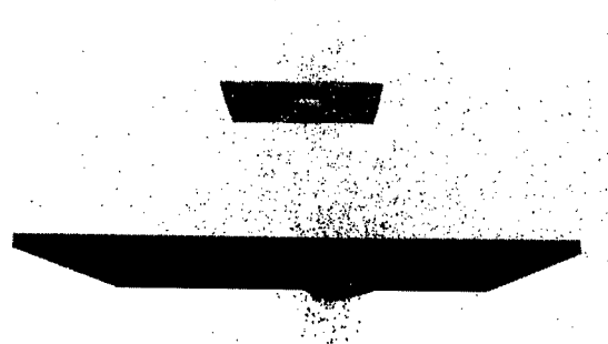
Fig. 2. Oblique Whipple shield impact simulation (t = 30.7 microseconds).
