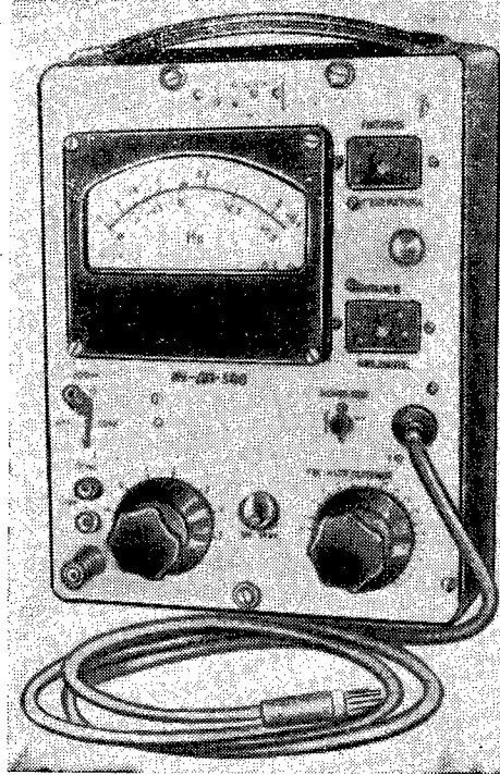
Figure 12.5.1. Exterior view of the IU-DP-300 remotely powered level meter.
