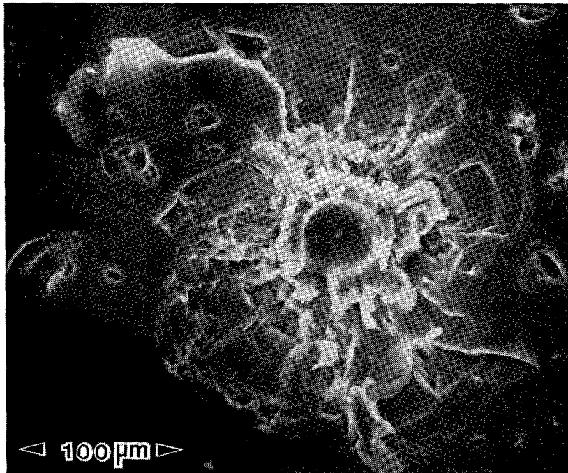
Figure 1: Scanning electron micrograph of impact in Zerodur displaying melt crater formation.
