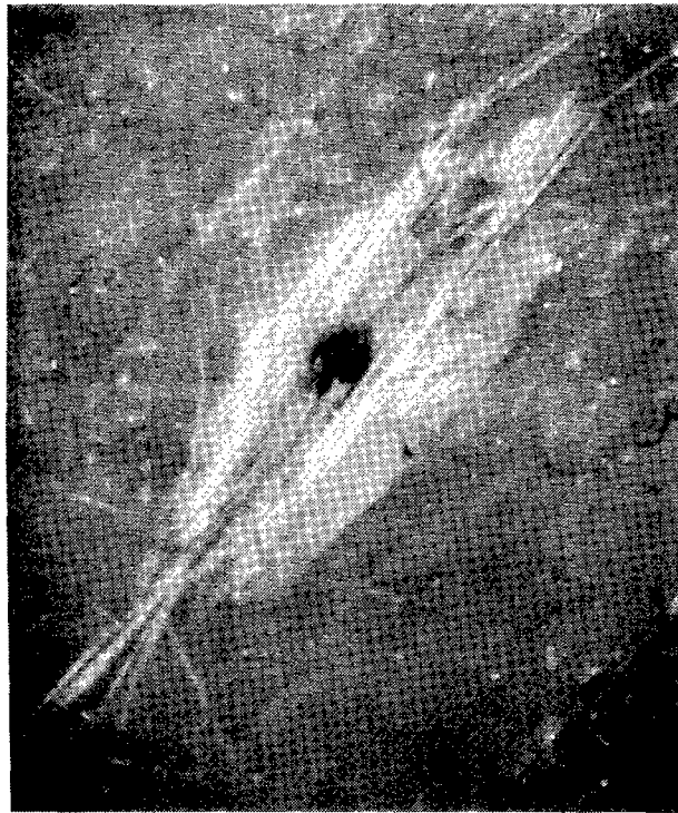
Figure 12. Micrometeoroid/debris impact damage ( \times 100 ) on Kevlar ® /epoxy tube [SP-328, ( \pm 45^\circ ) 4s ]
