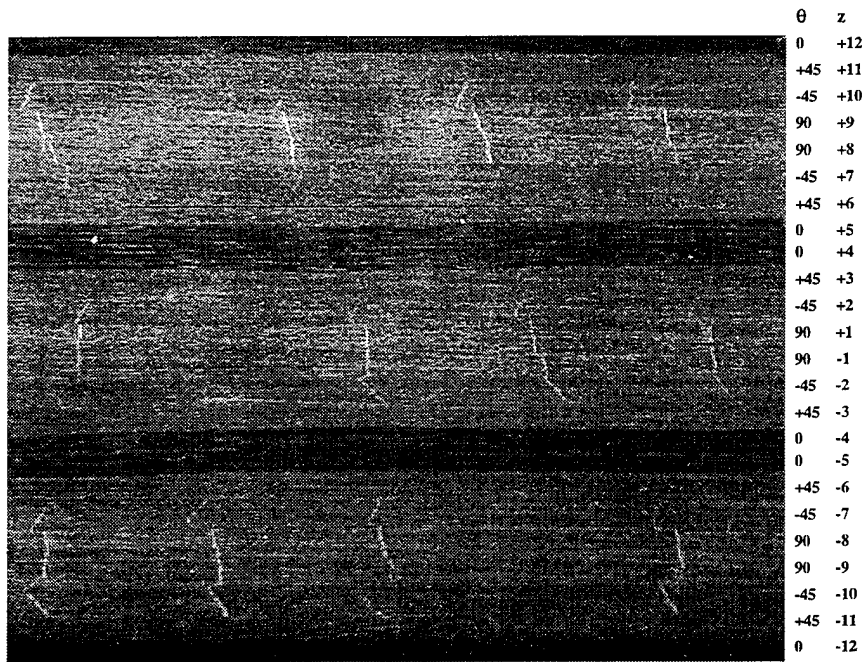
FIGURE 2. PHOTOMICROGRAPH OF [0/45/-45/90]_{s3} LAMINATE SHOWING PLY CRACKS
