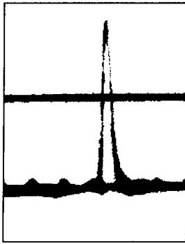
Fig. 5. Current derivative oscillogram of storage (L474-2) is 10^{12} A/s. Time marks are 2 \mu s.
