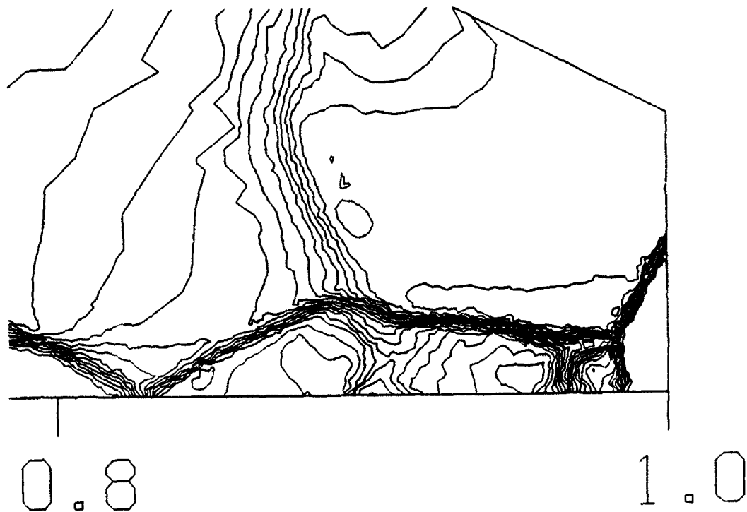
Figure 9a. Secondary Mach Reflection in a planar channel. Density contours.
