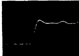
Shock Response from Accel-compensated Transducer
