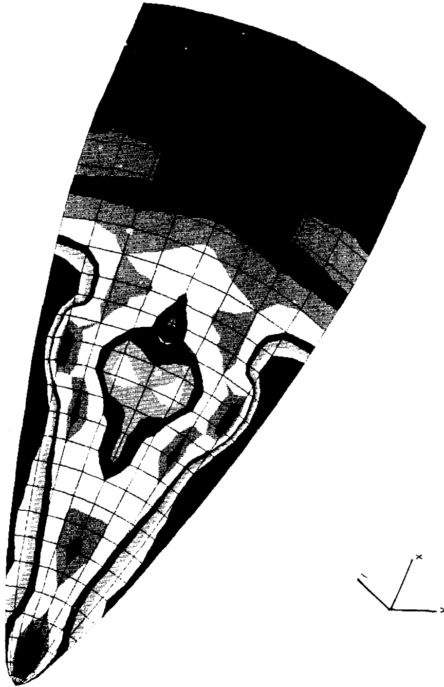
Figure 57. Inside shell surface first principal stresses at t = 6.2642 ms (step 18).
