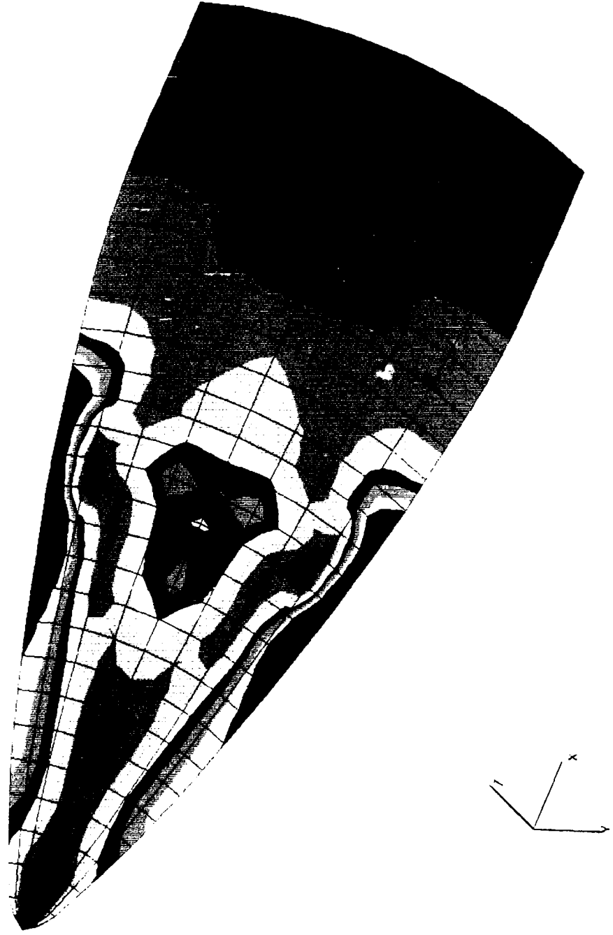
Figure 56. Inside shell surface first principal stresses at t = 4.7335 ms (step 14).
