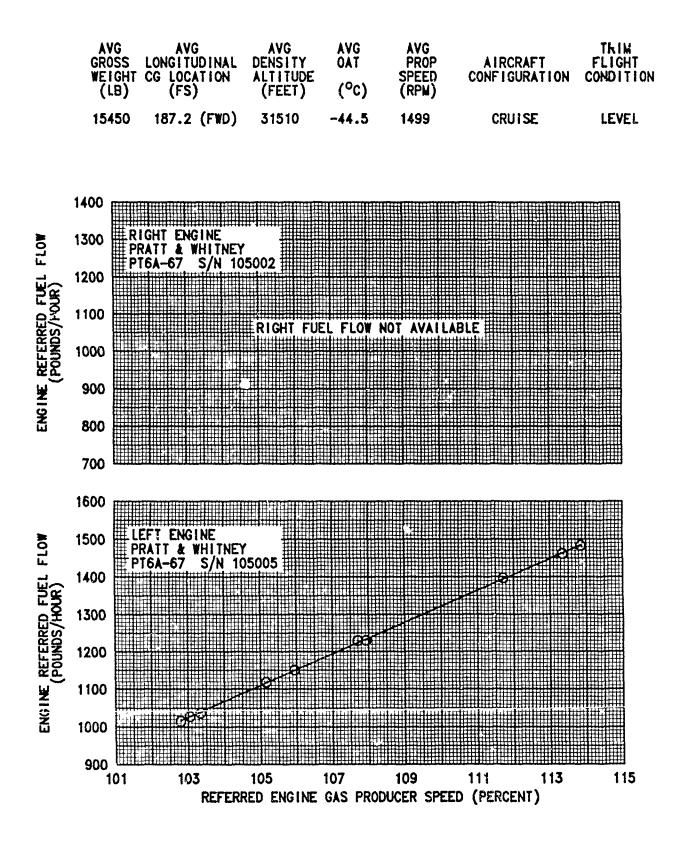
FIGURE E-5 ENGINE CHARACTERISTICS RC-12K USA S/N 85-50149
