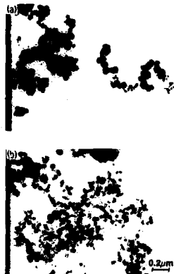
FIG. 1. TEM of ferrites formed from solutions with [Me]_{tot} = 0.25M and [N_2H_4]/[Me]_{tot} = 1.33 (a) and 5.33 (b).
