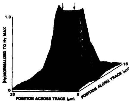
FIG. 3. Example of measurement of H_y along x at various positions across the track. The example shown is for a narrow-track head with a trackwidth of 8 \mu\text{m} and a pole-tip thickness of 3 \mu\text{m} . The arrows indicate the extent of the region of uniform H_y across the track.
