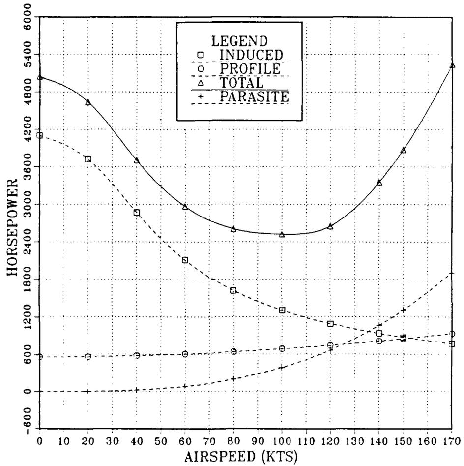
Figure A.4 Power versus Airspeed Plot
