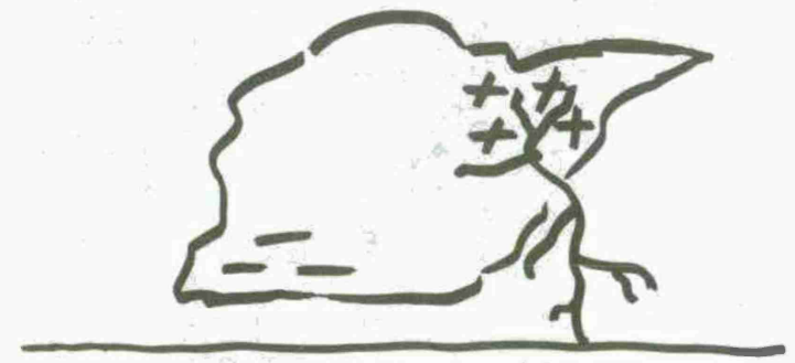
FIG 2b. TYPICAL DISCHARGE IN WINTER STORMS- POSITIVE STROKE.
