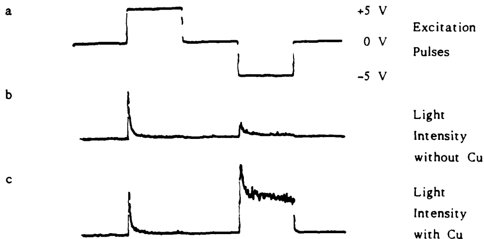
Fig. 1. Electroluminescence at anodized aluminium electrode.
