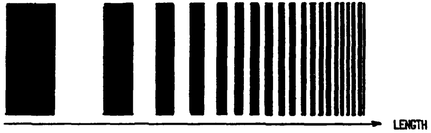
(A) SERIES OF LINES AND SPACES REPRESENTING INCREASING SPATIAL FREQUENCY
