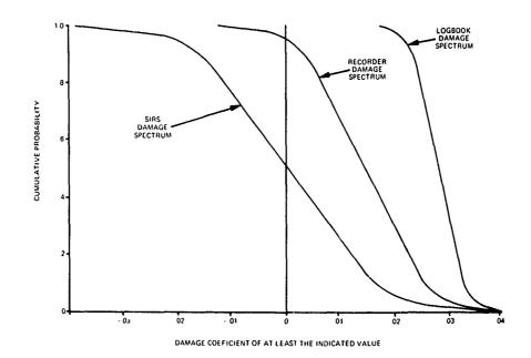
Figure 35. Main Rotor Yoke Extension Damage Spectrums.
