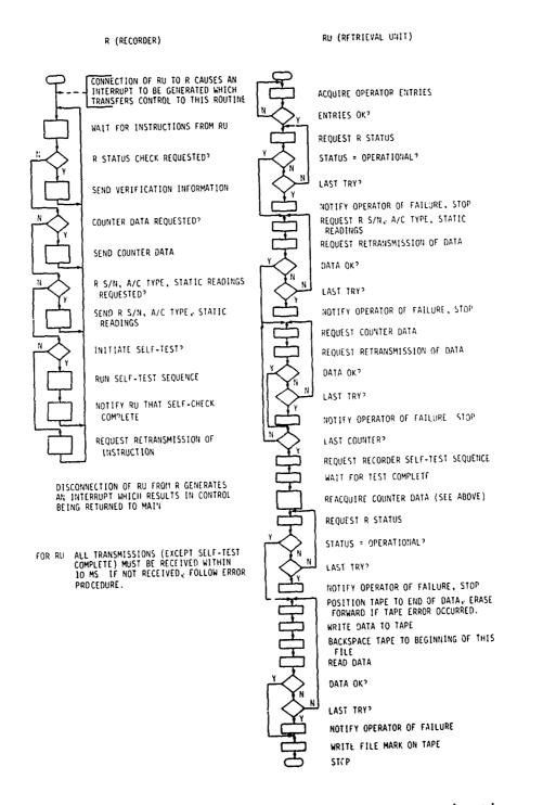
Figure 26. Retrieval Unit Recorder Communications.
