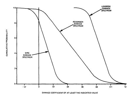
Figure 34. Main Rotor Blade Damage Spectrums.
