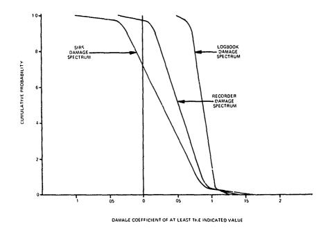
Figure 43. Tail Rotor Blade Damage Spectrums.
