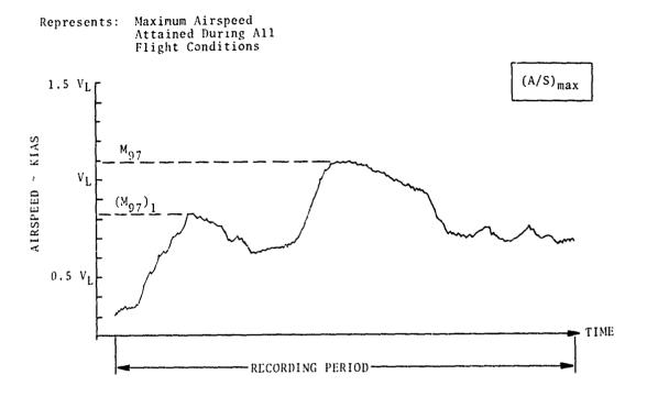
M<sub>97</sub> = maximum airspeed magnitude recorded during prescribed period (M<sub>97</sub>)<sub>1</sub> = intermediate maxima whose airspeed values were subsequently surpassed during the recording period
