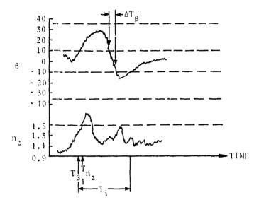
$T_i$  = asymmetrical pullup occurrence timer for FCC #i, i = 41,52  $T_{\beta i}$  = time at which roll attitude first exceeds 10° threshold  $T_{n_z}$  = time at which  $n_z$  exceeds 1.5 g threshold  $\Delta T_{\beta}$  = time between roll attitude threshold exceedances
