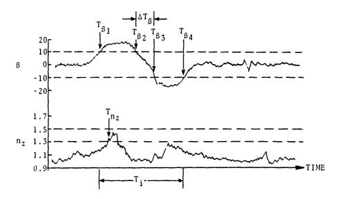
$T_{\beta 1}$  = time at which roll attitude first exceeds 10° threshold  $T_{\beta 2,3,4}^{\beta 1}$  = respective times at which roll attitude crosses 10° threshold
