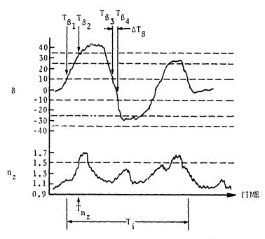
$T_{63,4}$  = second and third times the roll attitude crosses the 10° threshold level
