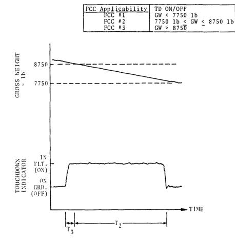
$\begin{array}{rcl} T_1 &=& FCC & \#1 & Timer \\ T_1 &=& FCC & \#2 & Timer \\ T_3^2 &=& FCC & \#3 & Timer \end{array}$
