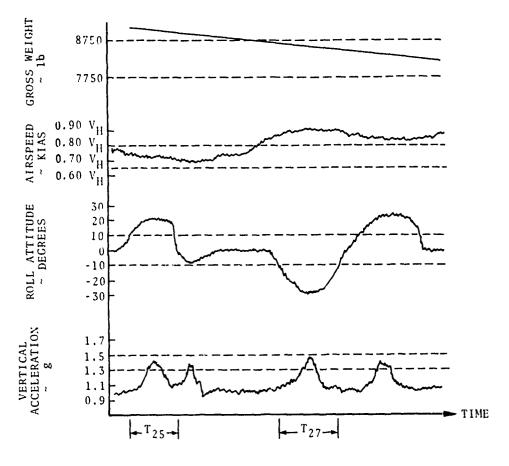
Figure A-8. Flight Condition Categories 23 through 28 (Normal (High-Speed) Turns).
