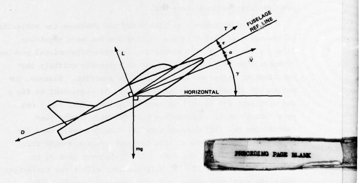
Fig. 1 Forces and Angles in Vertical Plane when Bank Angle Equals Zero
