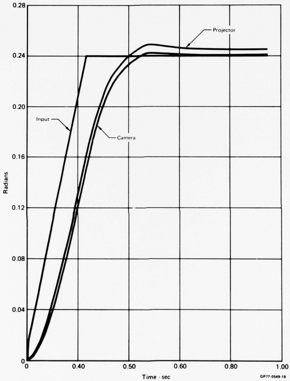
Figure 49 System Response for Stick Input Lag = 0.12 Sec
