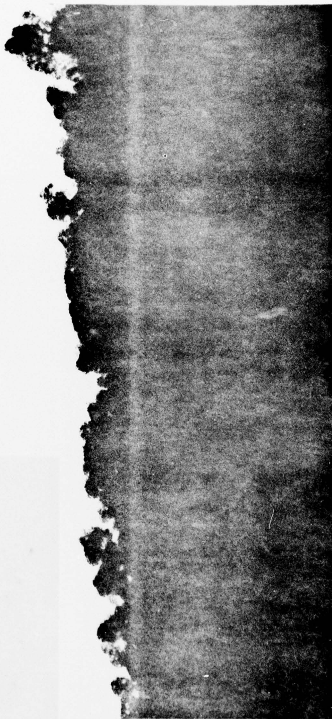
FIG. 37 PROFILE VIEW OF FP-IV FIBER EXTRACTED FROM Al-Li ALLOY MATRIX AND ELECTRON DIFFRACTION PATTERN OBTAINED FROM FIBER SURFACE. MATERIAL PROTRUDING FROM SURFACE IDENTIFIED AS LITHIUM SPINEL
