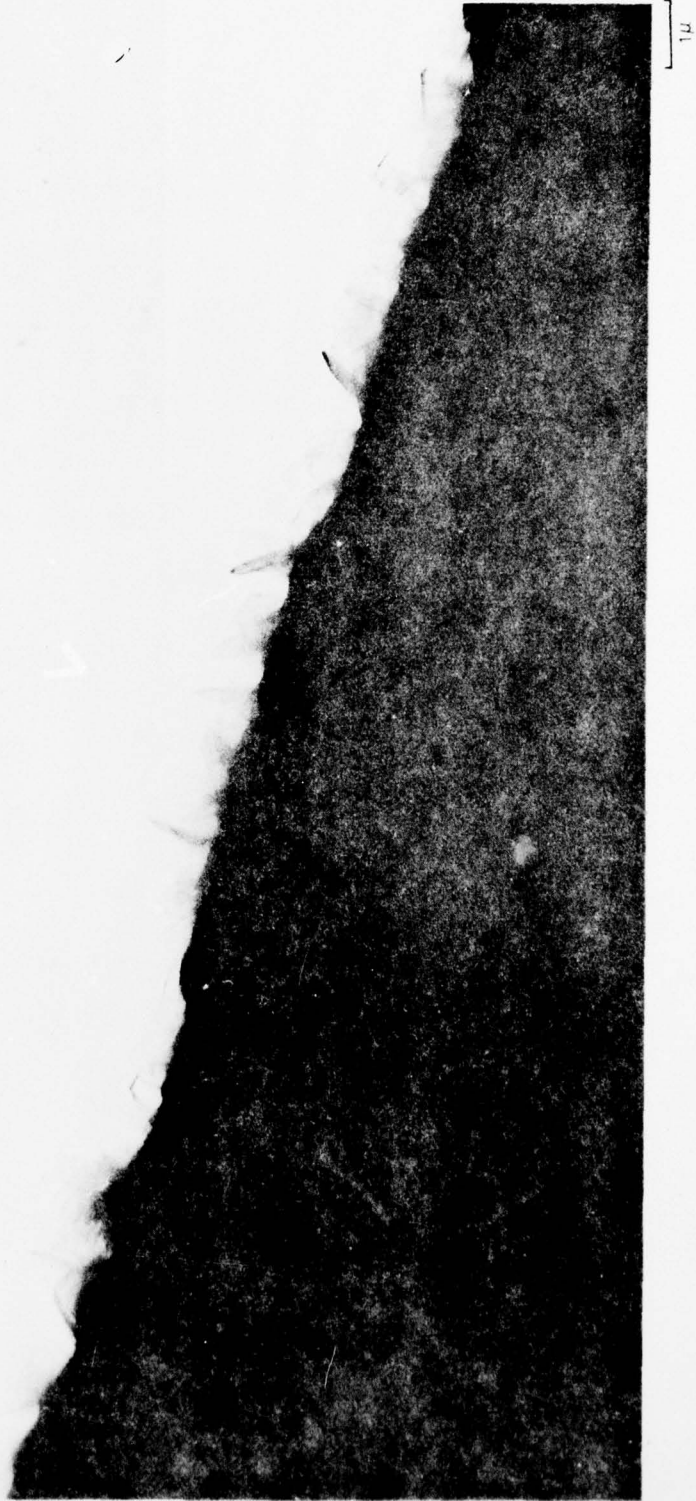
FIG. 38 PROFILE VIEW OF FP-IV FIBER EXTRACTED FROM Al-Li ALLOY MATRIX AND ELECTRON DIFFRACTION PATTERN OBTAINED FROM SMALL SINGLE CRYSTAL PLATELETS WHICH WERE A MINOR (5%) SURFACE CONSTITUENT
