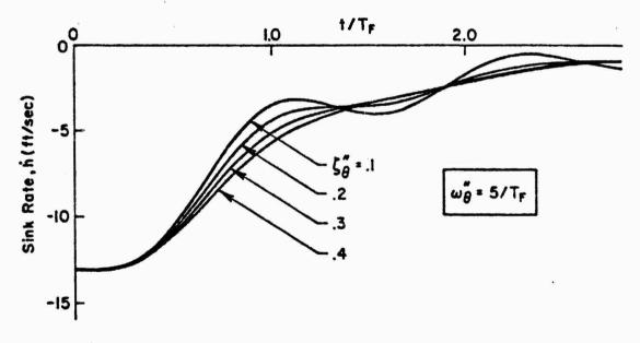
b) Effect of Closed Loop Path Mode Damping Ratio on Flare
