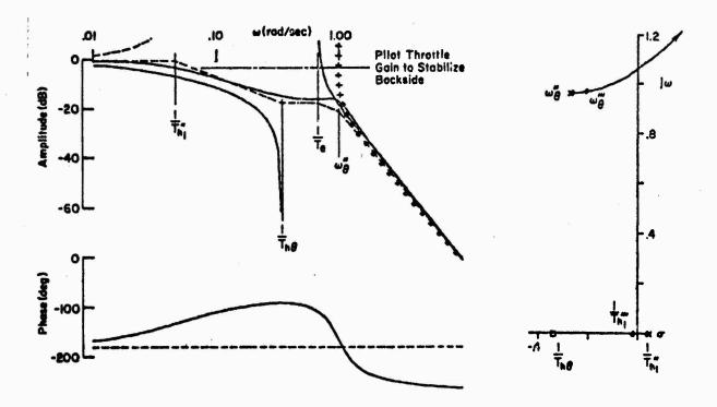
Figure 25. Use of Secondary Control to Stabilize Backside Mode Generic Configuration BSL1
