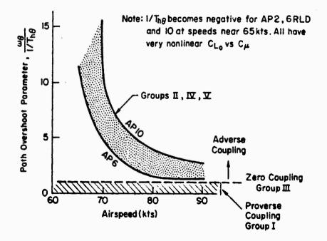
Figure 7. Effect of Airspeed on the Dynamic Response
