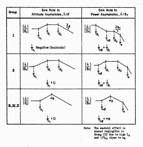
Figure 6. Generic Characteristics for Sink Rate Control with Attitude and Throttle
