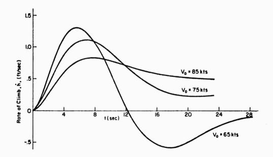
Figure 8. Effect of Speed on Path Response to a Unit Step Fower Input (AP10)
