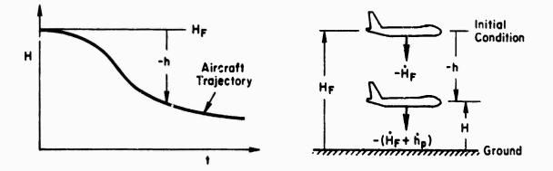
Figure B-1. Relationships Between Inertial and Perturbation Coordinates
