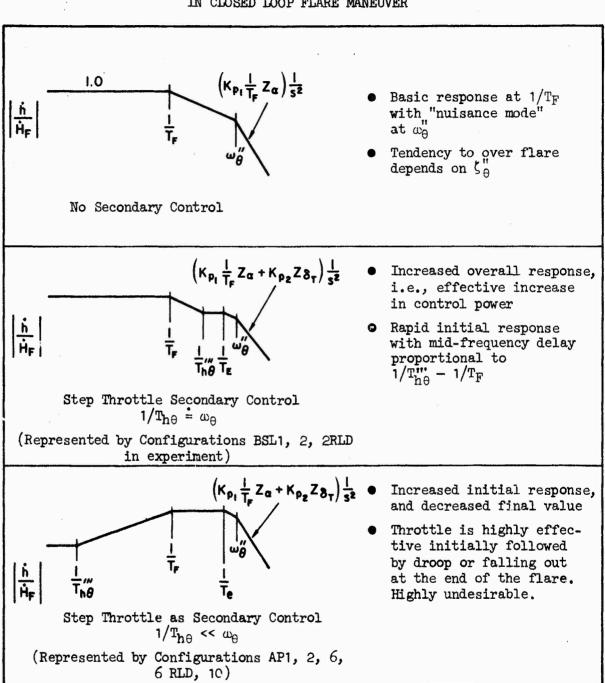
EFFECT OF THROTTLE STEP AS SECONDARY CONTROL IN CLOSED LOOP FLARE MANEUVER
