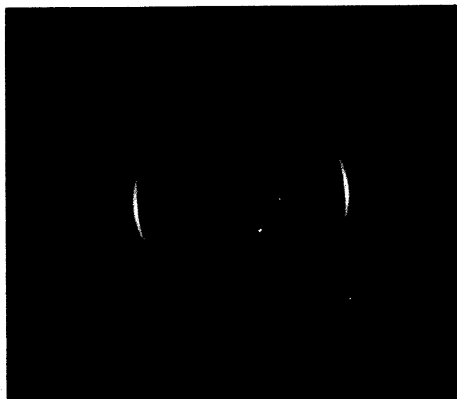
Wide Angle X-Ray Diffraction Pattern of PE
