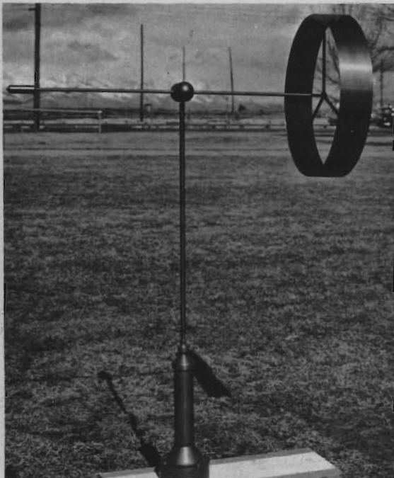
(A) An annular fin bivane used at the National Reactor Testing Station
