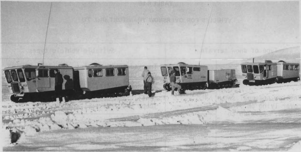
Figure 8-36. Polecat Train in Greenland (Front and rear tractors in this train have power units in front portion of articulated carrier. Center tractor has power unit in rear portion of articulated carrier.) (Photograph by R. W. Gerdel)
