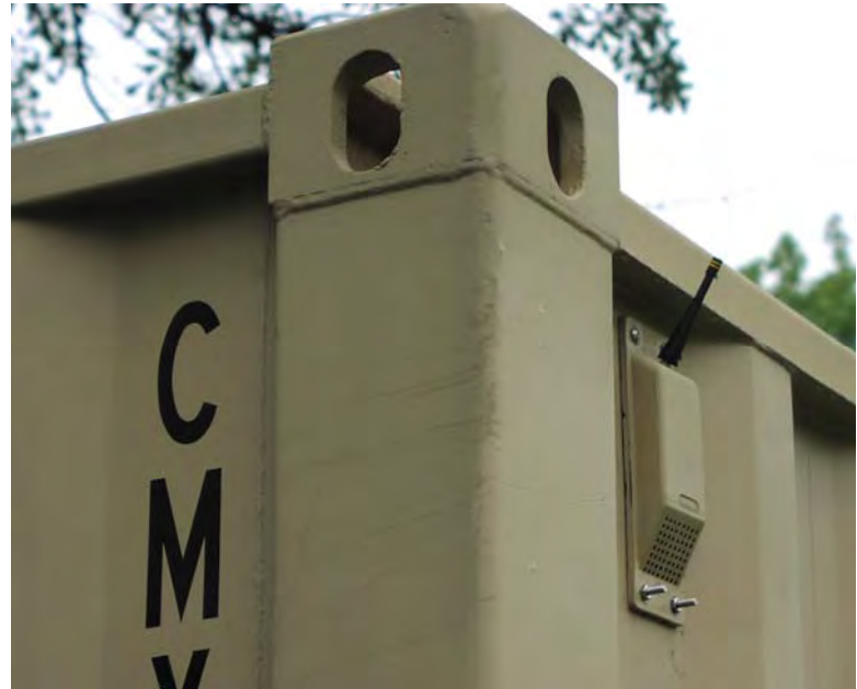
USMC TRICON with prototype Integrated Sensor / RFID
