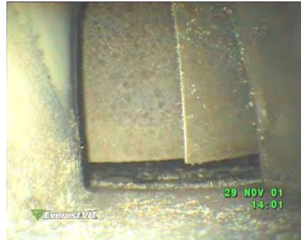
Corrosion Inside TF-34 Engine (S-3)
