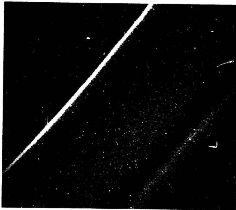
Fig. II.14. (a) An extreme example of a guide with rough walls and top surface. (The guide is 3\mu high and 7\mu wide.) (b) Good quality channel waveguide fabricated by using holographically prepared mask and ion polishing. (The guide is 1.4\mu high and 2\mu wide.)
