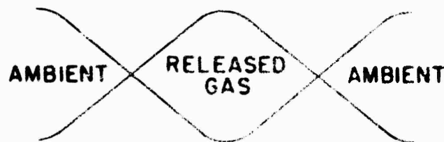
Figure 1. Model of Density Profile of Released Gases and Ambient
