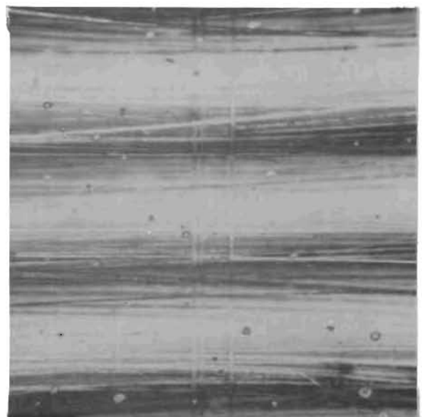
Figure 140. Test Model F, Seat, 0.0065- x 0.0065-Inch Interference Photo With-Lay Showing 0.0005-Inch Radius Profilometer Stylus Scratches
