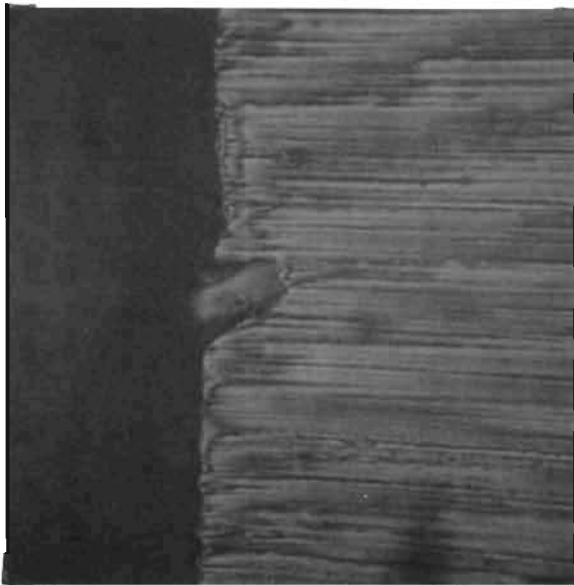
Figure 123. Test Model D f , Seat, 0.0065- x 0.0065-Inch Interference Photo at OD Showing Fracture
