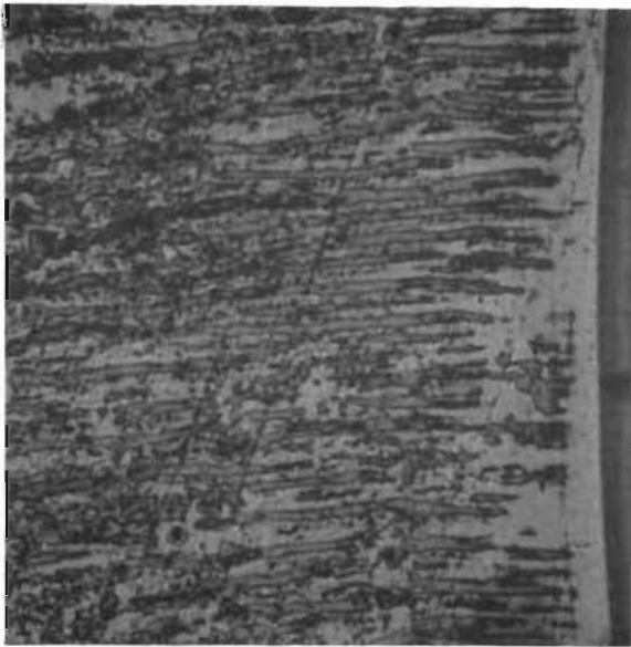
Figure 153. Test Model G_{f1} , Seat, 0.0065- x 0.0065-Inch Plain Photo Showing Corrosion Fretting Before Wiping at ID
