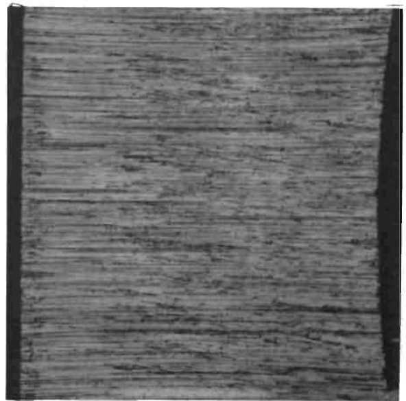
Figure 124. Test Model D f , Seat, 0.033- x 0.033-Inch Plain Photo Showing Corrosion Fretting After 91,800-psi Cycle Test
