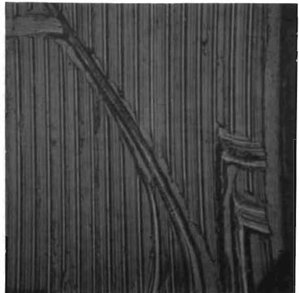
Figure 116. Test Model R_f , Seat, 0.0065- x 0.0065-Inch Plain Photo Showing OD Plastic Deformation at Right and Handling Scratch
