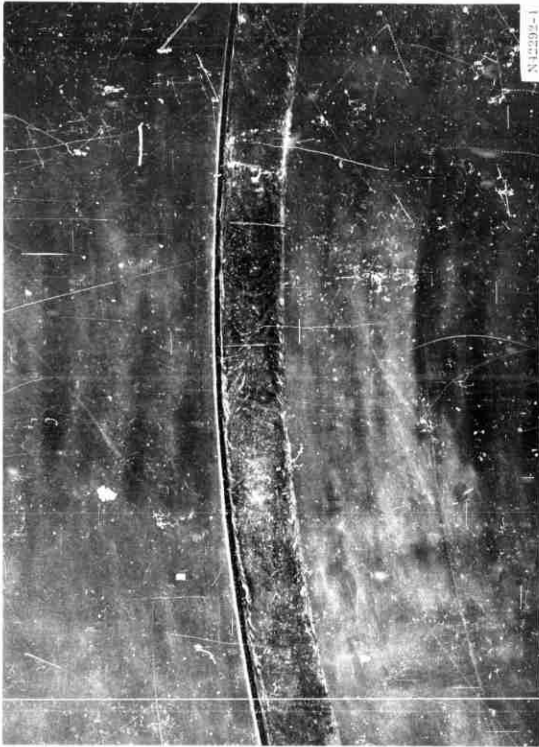
Figure 88. Slot Former Support Ring after Plaster Mold Removal
