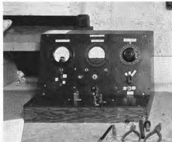
FIGURE 31. Rectifier filter test position (Bowen).
