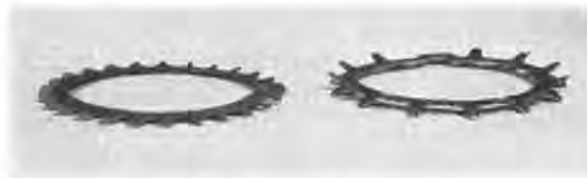
FIGURE 49. Washers used for mounting fuzes in bombs. Lock washer is shown on the left, nonlocking spring washer on the right.
