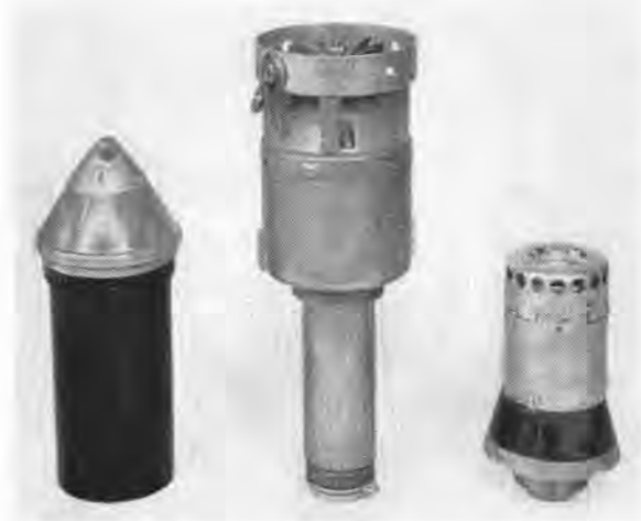
FIGURE 4. Radio proximity fuzes for rockets. These are from left to right: (1) T-5 fuze for 4.5 in. M-8 rocket for air-to-air use (T-6 ground-to-ground fuze is identical in appearance to T-5); (2) T-2004 fuze for 5-in. AR rocket for air-to-ground use; and T-2005 multiple-purpose fuze.
