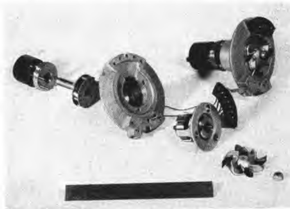
FIGURE 23. Power supply and arming system for T-82 fuzes.
