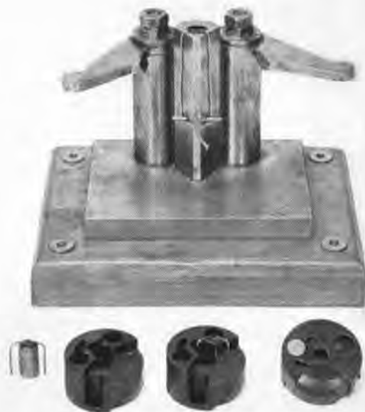
FIGURE 40. Jig for forming and cutting detonator leads in mortar fuzes. At bottom of photograph are shown from left to right: detonator, detonator rotor, detonator rotor with detonator installed, bottom view of detonator rotor showing lower face of detonator.
