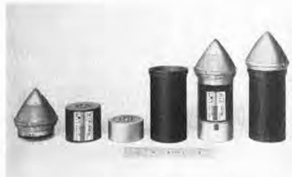
FIGURE 12. T-5 fuze, components and assembly. From left to right: electronic assembly designated as MC-382; battery power supply designated as BA-75; arming switch designated as SW-200; housing which contains tetryl booster; partial assembly of fuze; fuze completely assembled ready for installation in rocket.
