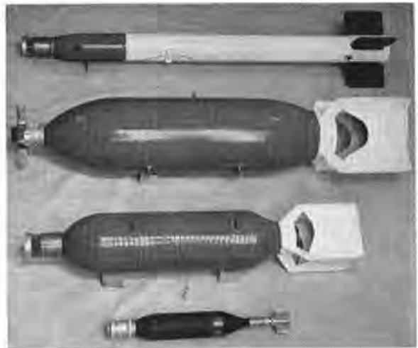
FIGURE 7. Radio proximity fuzes on typical missiles. These are, from bottom to top: (1) T-132 fuze on 81-mm M-56 mortar shell; (2) T-91 fuze on M-81-A 260-lb fragmentation bomb; (3) T-51 fuze on the M-64, 500-lb general purpose bomb; and (4) T-2004 fuze on 5-in. HVAR rocket.
