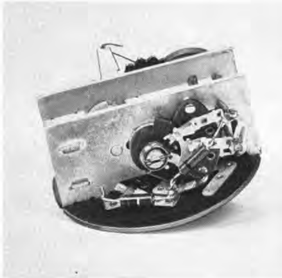
FIGURE 11. Impact detonator for T-6 fuze.
