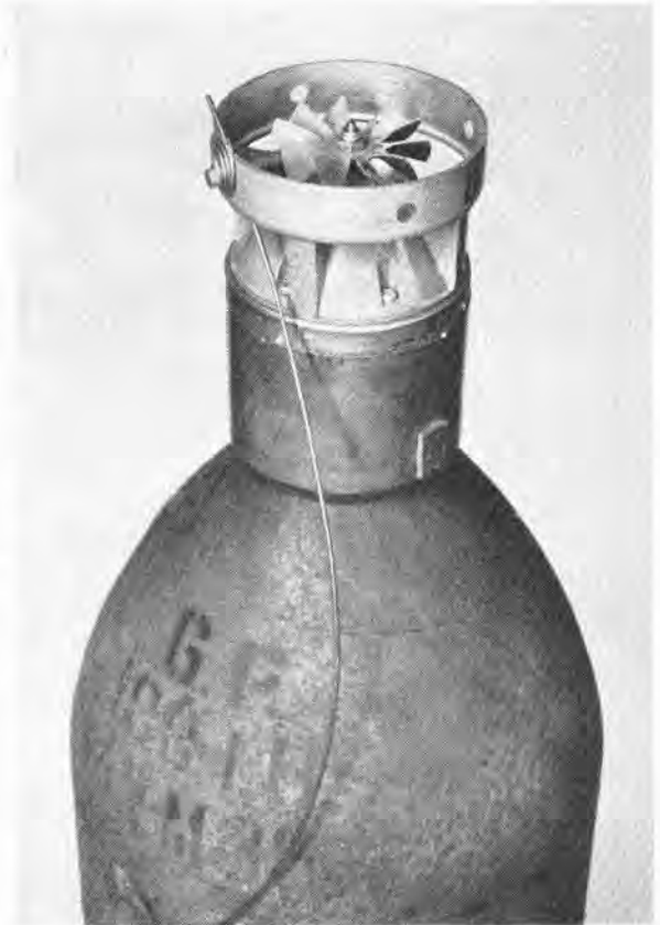
FIGURE 20. Use of arming wire and locking pin to prevent vane rotation.
