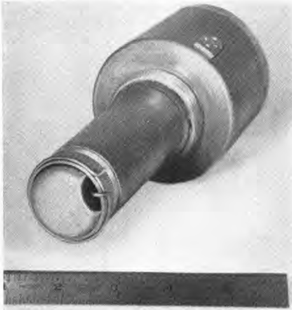
FIGURE 23. Safety pin installed in T-50 type fuzes. Pin is removed before fuze is inserted in fuze well.
