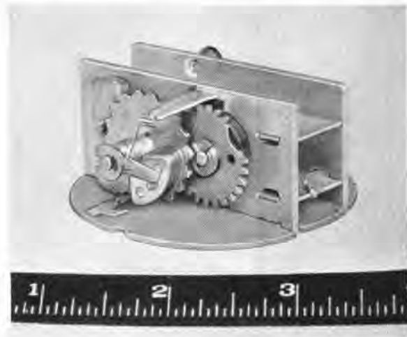
FIGURE 10. Self-destruction element for T-5 fuze.
