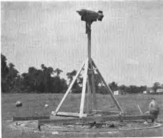
FIGURE 18. Rotatable platform holding fuze bomb for directivity pattern measurements.
