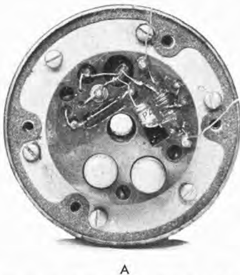
FIGURE 15. RGD circuit for T-51 fuze. A is photograph of oscillator block. B is circuit diagram arranged to correspond to photograph.
