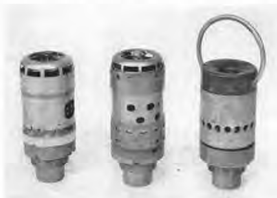
FIGURE 6. Radio proximity fuzes for trench mortar shells. These are, from left to right: (1) T-132 fuze using electric circuits "printed" on ceramic plates; (2) T-171 fuze, electrically similar to T-132 but with standard electrical resistor and condensers; and (3) T-172 fuze with loop antenna.
