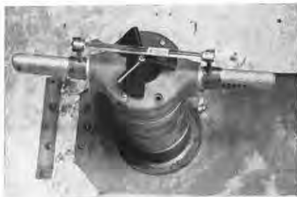
FIGURE 7. Resistor for determining sensitivity of bar-type fuzes.
