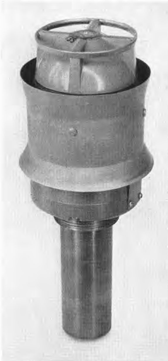
FIGURE 48. Experimental model of generator-powered fuze for air-to-air bombing.
