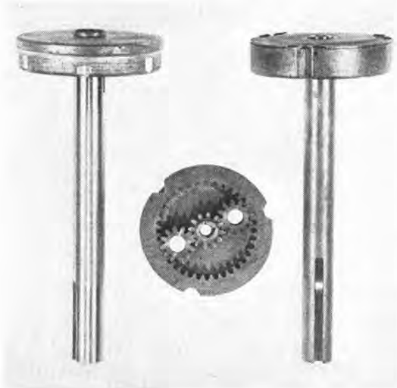
FIGURE 21. Planetary-type speed-reducing device for T-50 fuzes.
