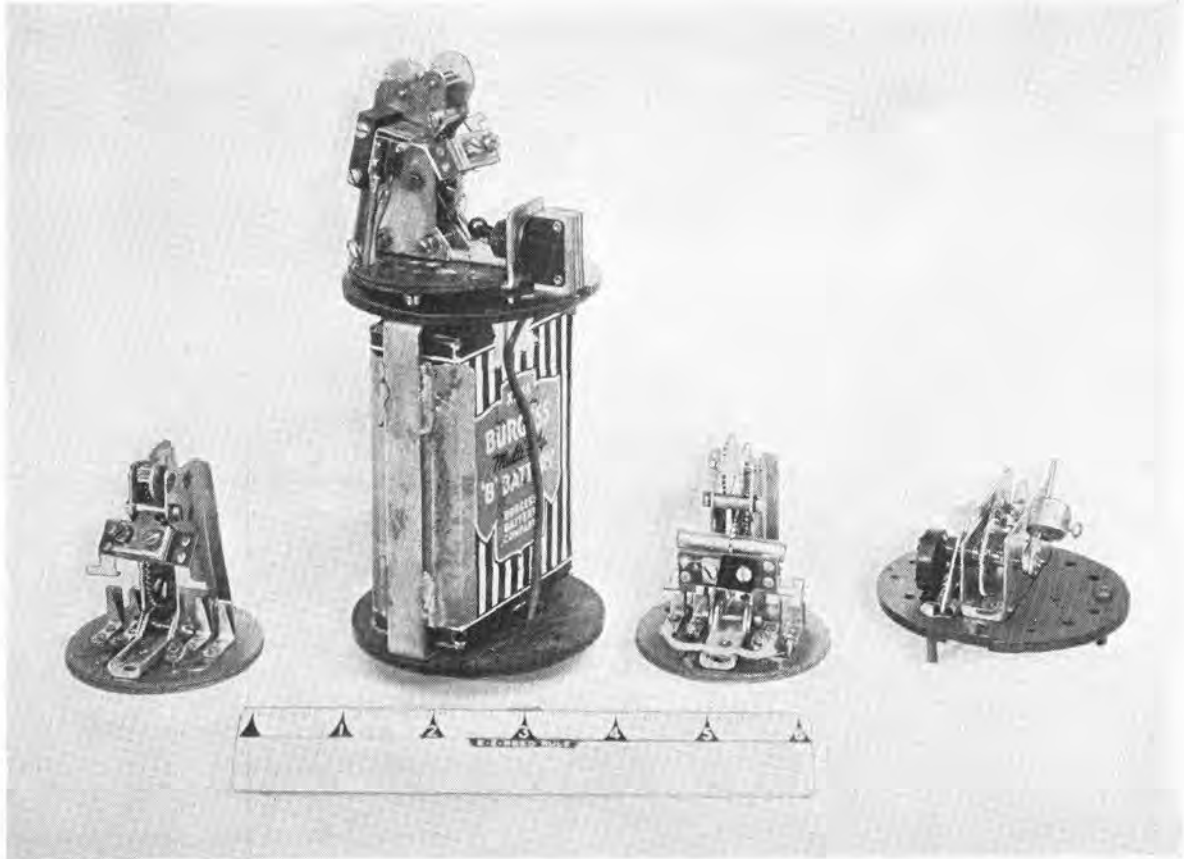
FIGURE 4. Acceleration-operated arming device. This is a British design developed for use on their rocket fuzes.
