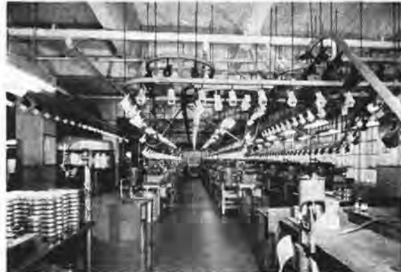
FIGURE 33. Assembly line for radio proximity fuzes showing overhead conveyor for moving completed fuzes to final test position (Emerson photograph).
