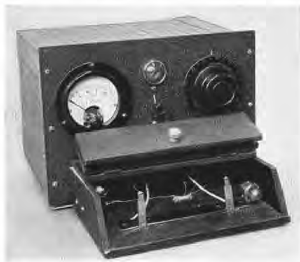
FIGURE 17. High potential leakage tester. Double-wound coil for T-51 fuze is shown being tested for insulation between coils.
