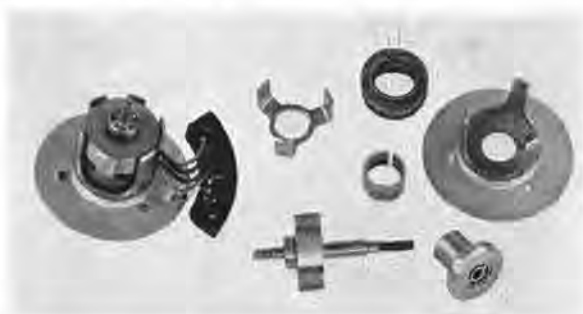
FIGURE 71. T-82 generator and principal components. Assembled generator is shown at left. Grouped at right are spider, coil, core, rotor, center stud with upper bearing, cup with cover plate.
