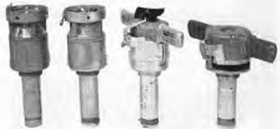
FIGURE 5. Radio proximity fuzes for bombs. These are, from left to right: (1) T-50-E1 fuze for air-to-ground use on M-30 and M-81 bombs; (2) T-91 fuze, a later and improved version of T-50-E1, for use on M-30, M-81 and M-64 bombs; (3) T-51 fuze, air-to-ground use, for use on all bombs of 100-lb size or larger; and (4) T-82 fuze for use paralleling T-51.
