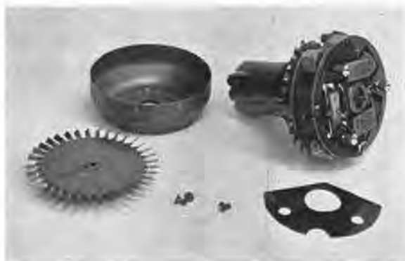
FIGURE 72. P-4 power supply, partly disassembled. Stator and its two armature coils can be seen at right edge of generator assembly. (Photograph by Bell Telephone Laboratories.)
