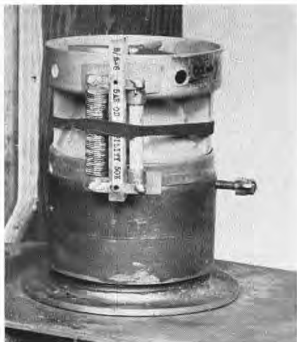
FIGURE 3. Compensated loading resistor on ring-type fuze.
