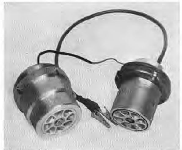
FIGURE 13. Reference vibration heads used to calibrate vibration response of test fixtures.
