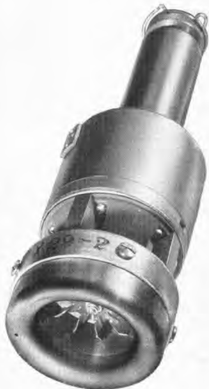
FIGURE 30. Doughnut arming device installed in fuze.
