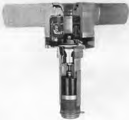
FIGURE 58. Fuze T-82 with section cut away. Central air duct to turbine can be seen. Generator was immediately below and directly coupled to turbine.
