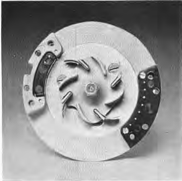
FIGURE 63. Turbine mounted on base assembly of bomb fuze, T-82.
