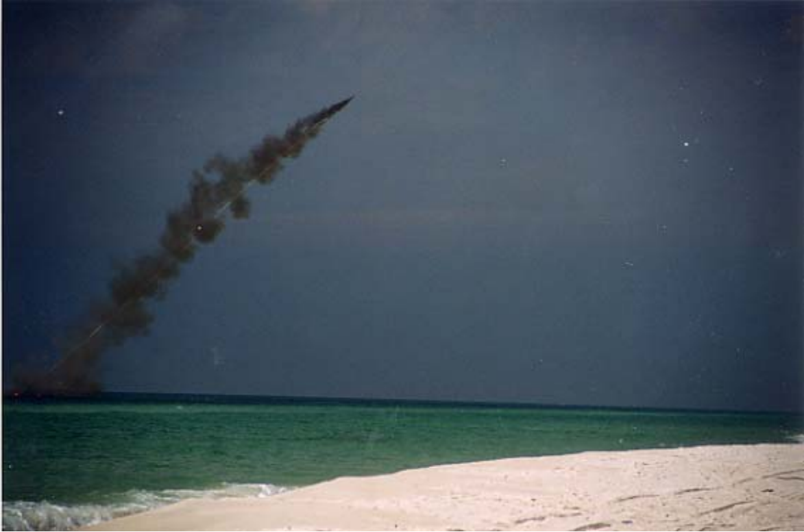
Figure 2-3. Line Charge Fired from Amphibious Assault Vehicle (AAV) in the Gulf of Mexico Towards SRI
