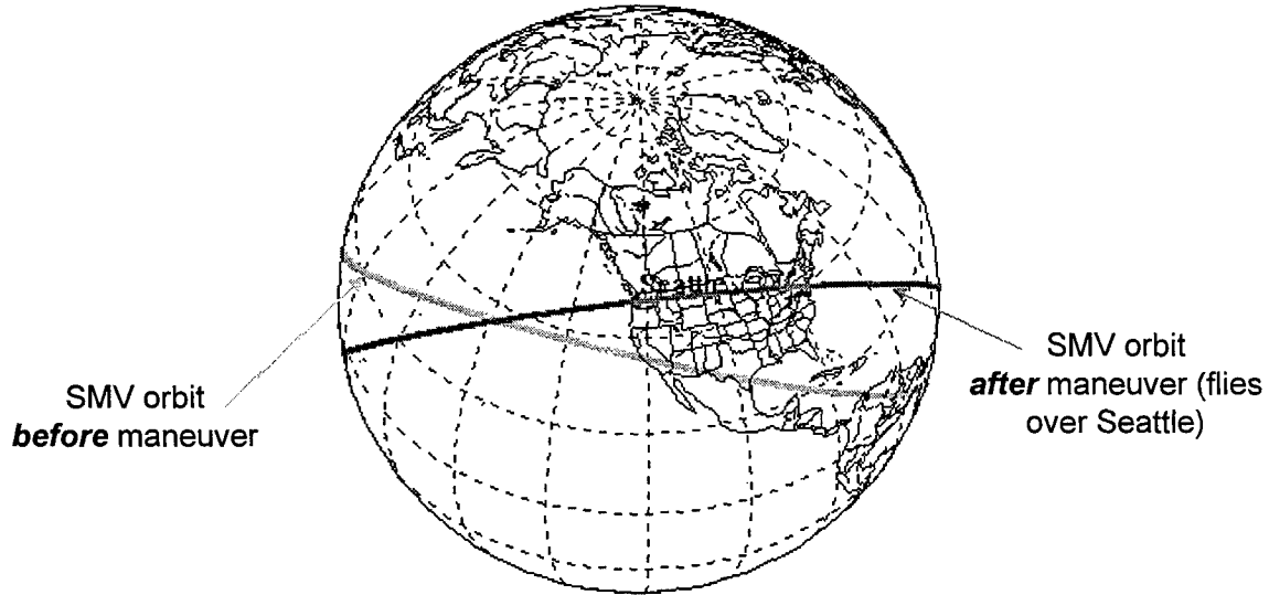
Figure 14 Satellite Tool Kit (STK) orbital simulations before and after maneuver for Program Test 2 showing overflight of ground target (Seattle, WA)
