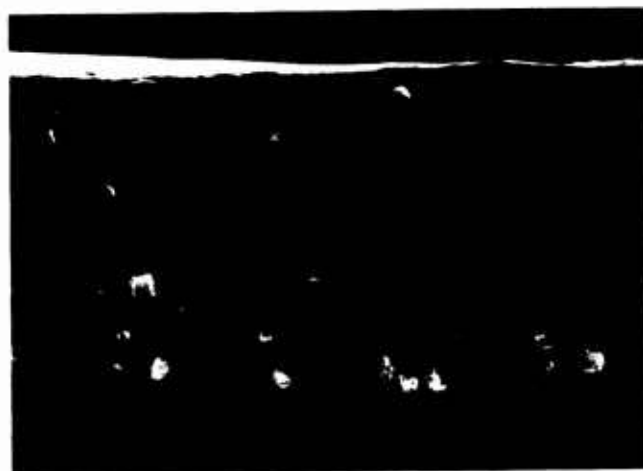
Fig. 2. Cross section of a DEF emulsion, imaged by a SEM. Sample sections were obtained by breaking liquid-nitrogen-frozen pieces of film. The average grain size was estimated from such photos by the measurement of the outermost embedded grains.
