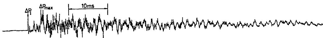
Figure 2 A pressure record taken at R_g position in the fully enclosed configuration, C1 (Data sampled at 20 microseconds per point or 50 KHz.)
