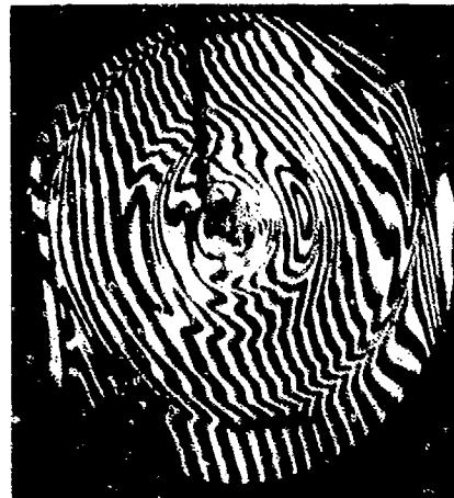
Fig. 2: Interferogram of the wave pattern generated by a PETN pellet in a PMMA plate.
