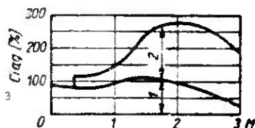
Fig. 10.3. Variation of compound engine thrust as a function of Mach number: 1) turbojet engine; 2) ramjet engine; 3) thrust (%).
