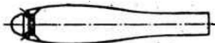
Fig. 7.19. Pulsejet engine with an inlet screen which reduces the effect of flight velocity on its performance.
