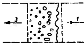
Fig. 6.4. Schematic diagram of the flame zone in the case of turbulent combustion of homogeneous mixtures: 1) mixture; 2) turbulent flame; 3) products of combustion.
