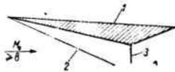
Fig. 8.43. Hypersonic ramjet engine with external combustion: 1) hypersonic flight profile; 2) oblique shock wave; 3) flame front.
