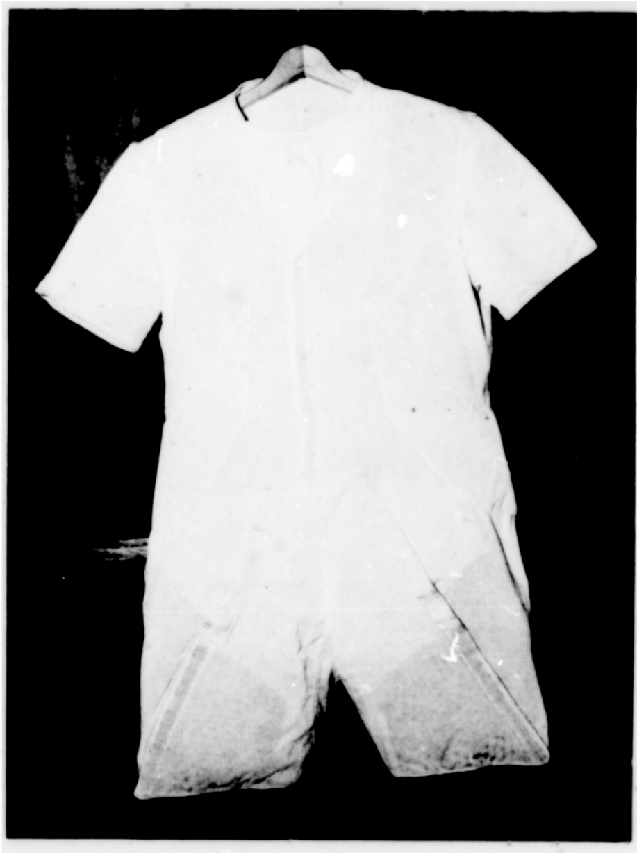
Fig. 22 NATICK AIR-COOLED SUIT, FRONT
