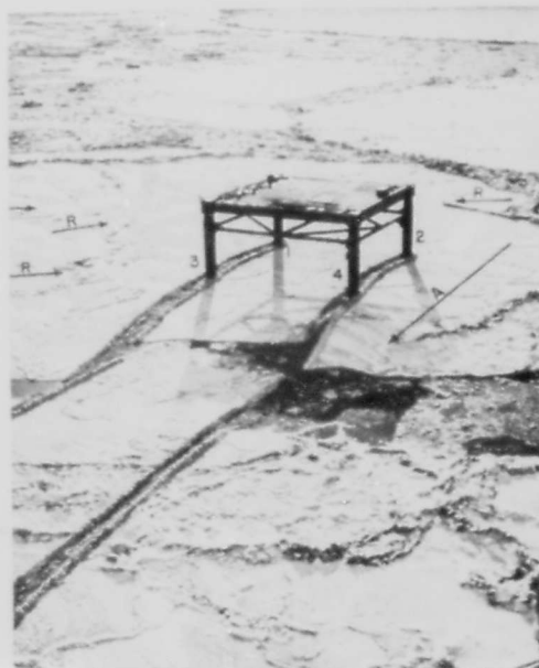
Ice Failure Against Platform, I, Note the Double Thick Rafted Section and the Small Flow Size.
