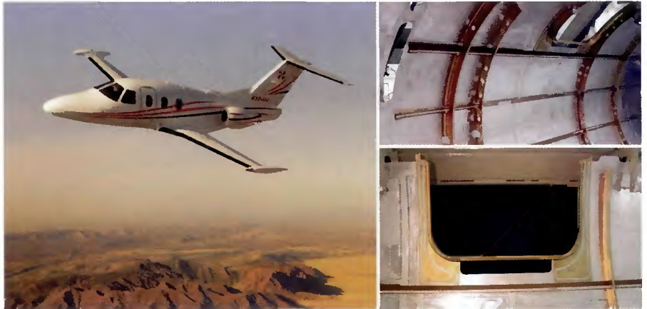
Fig. 7 — The Eclipse 500 business class jet is currently in final FAA certification trials (left). The internal longitudinal and circumferential aluminum stiffeners (right, top) and window and door doublers (right, bottom) are attached to the aluminum fuselage section with friction stir welded lap joints. Courtesy of Eclipse Aviation.
