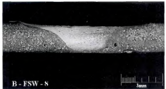
Fig. 16 — Cross section of a friction stir weld made on 2-mm vacuum cast AZ91 (left side is advancing side).
