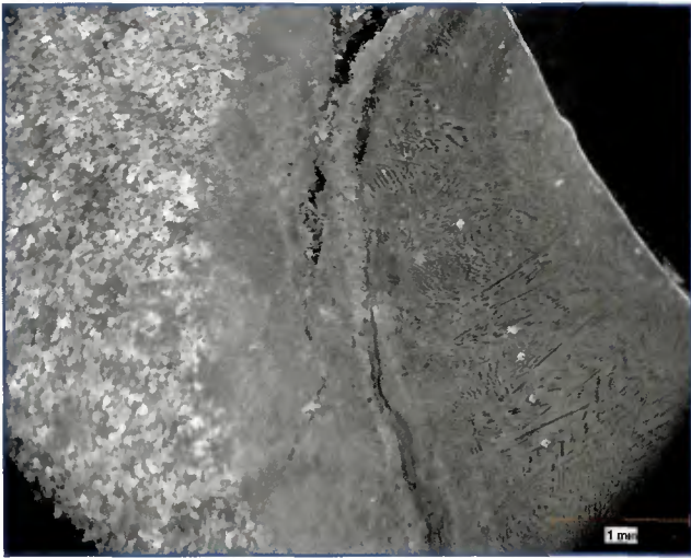
Fig. 2 — Heat-affected zone crack in gray cast iron welded to 304L with 312 filler metal.
