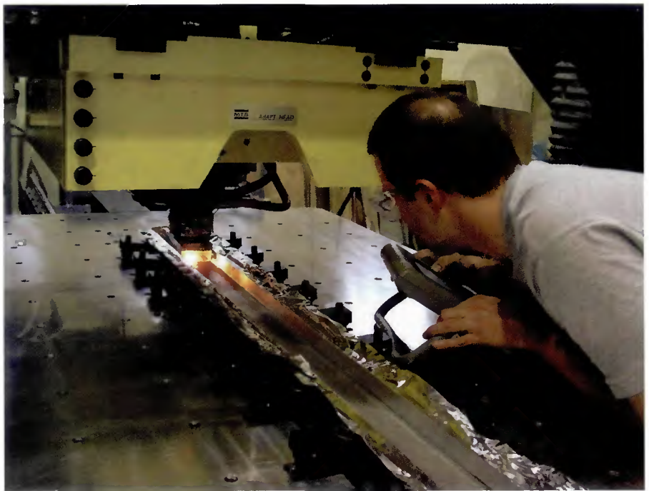
Fig. 11 — Joining of long lengths of contamination-free Ti-6Al-4V are possible with “out of chamber” friction stir welding using shrouds and trailing shoe shielding gas systems. Courtesy of Lockheed Martin Space Systems.
