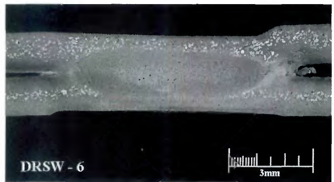
Fig. 4 — Cross section of 1.5-mm Thixomolded AM60 spot weld ( F = 4.0 kN, weld time = 6 cycles, weld current = 23 kA, downslope time = 4 cycles, downslope current = 23–16.5 kA).
