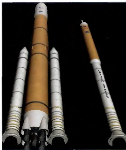
Fig. 6 — An artist's rendering of the Cargo Lift Vehicle (left) and the Crew Launch Vehicle (right).
