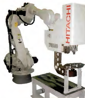
SWING-STIR Hitachi's unique Spot FSW machine
