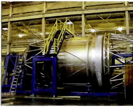
Fig. 2 — Circumferential weld tool for FSW with recently welded transition rings and dome.
