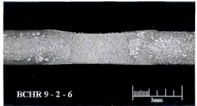
Fig. 8 — Cross section of a conductive heat seam weld made on 2-mm vacuum cast AZ91.
