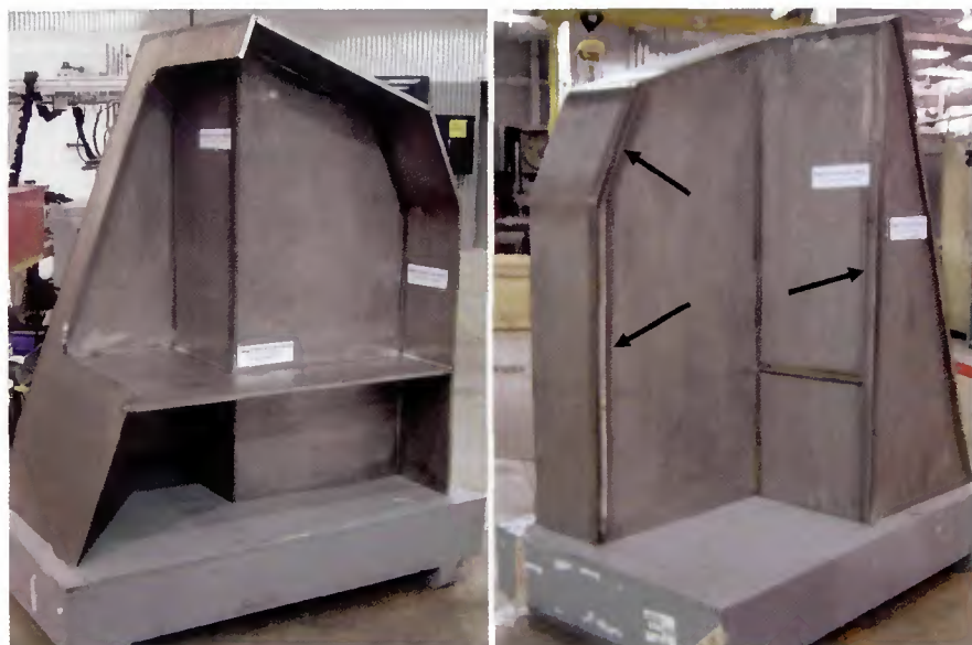
Fig. 2 — Edison Welding Institute used a combination of friction stir welding, GMAW, and hybrid laser beam welding to fabricate this demonstration article from thick-section titanium plates. FSW was used to join the 0.50-in.-thick plates in a corner joint configuration (arrows) to establish the basic shape of the article, and GMAW and hybrid laser beam welding were used to complete the assembly. Courtesy of Edison Welding Institute.
