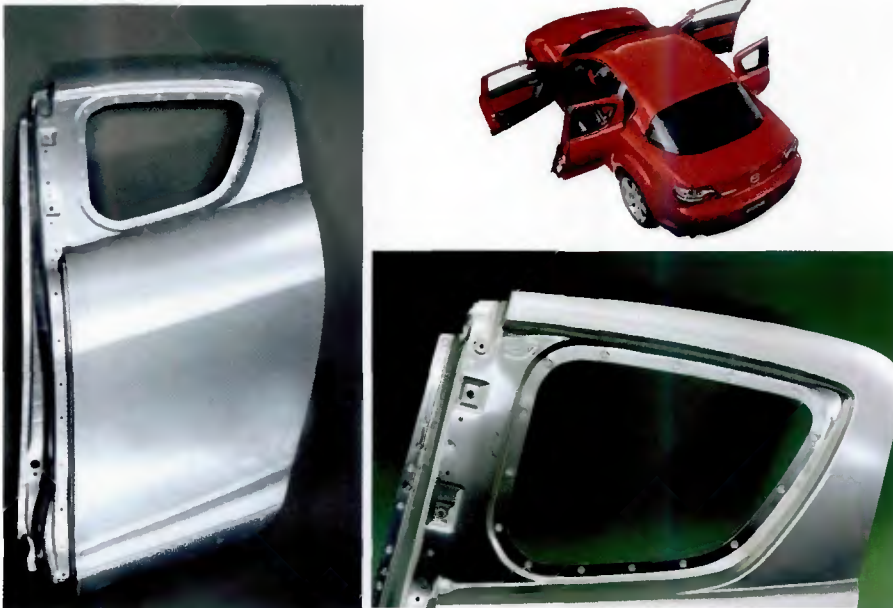
Fig. 13 — Use of the plunge friction spot welding (PFSW) method on the Mazda RX-8 rear door structure provides for structural stability against side impact and five-star rollover protection at reduced production costs. Courtesy of Mazda Motor Corp.
