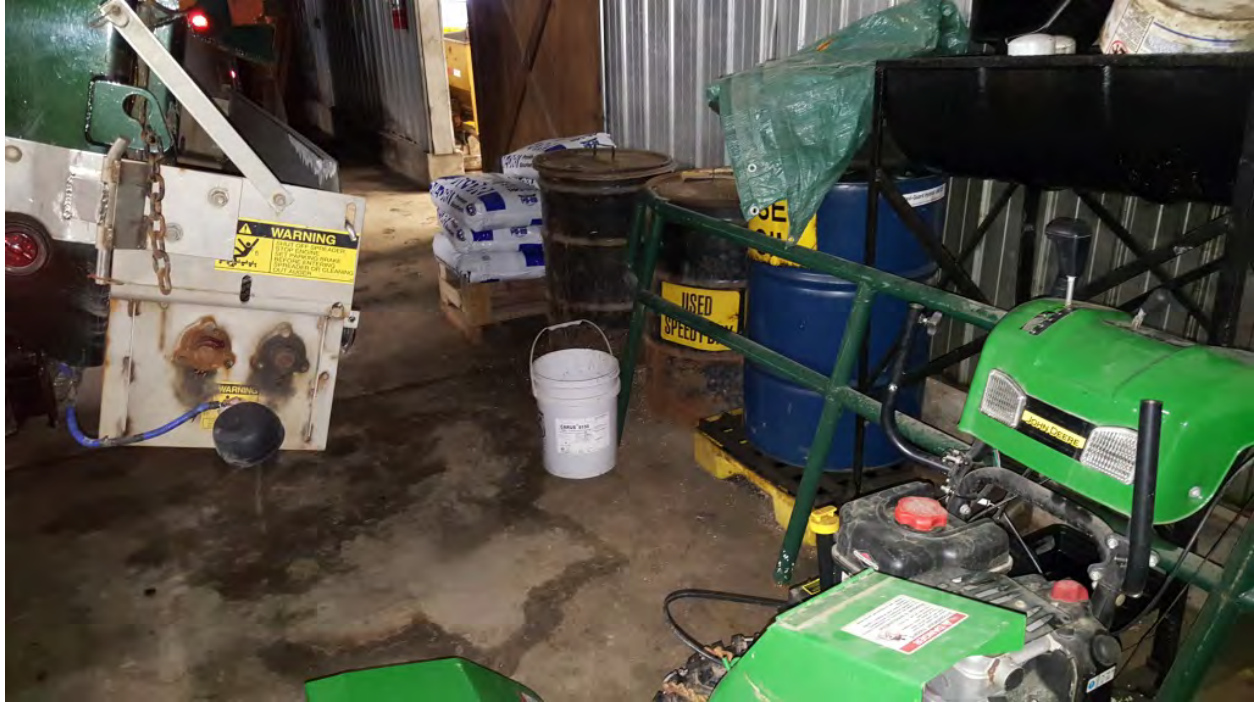
Photo 21: A drum of used oil on a spill containment pallet and a drum of used speedy dry. These items are located in the garage portion of the main DPW building.
