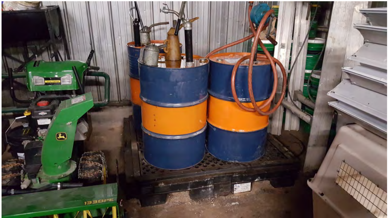
Photo 20: Drums of engine oil on a spill-containment pallet in the garage portion of the main DPW building.
