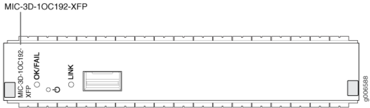
Figure 51: SONET/SDH OC192/STM64 MIC with XFP
