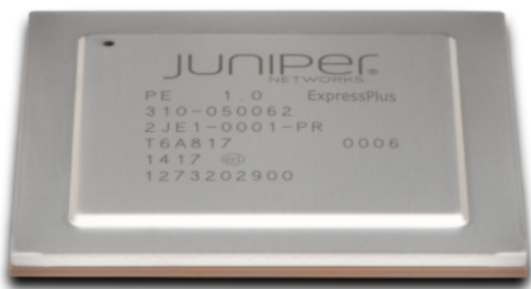
Figure 1: The custom-built Juniper Q5 ASIC
