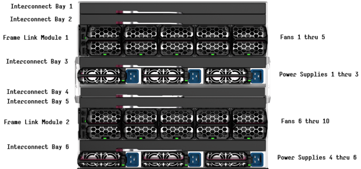
HPE Synergy 12000 Frame - Rear View
